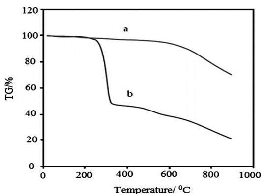
Fig. 8- The thermogravimetric curves of the MCN-1 (a) and MDA-MCN-1 (b) in nitrogen atmosphere [21].
