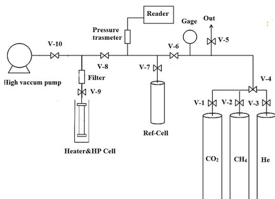
Fig. 3- Setup for gas adsorption capacity test.
