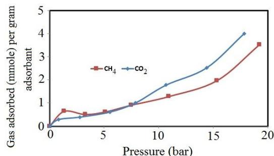
Fig. 9- CO<sub>2</sub> and CH<sub>4</sub> adsorption isotherms of MDA-MCN-1.
