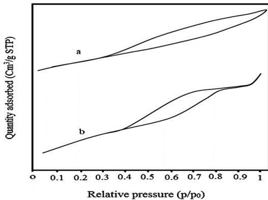
Fig. 5- Nitrogen adsorption-desorption isotherms for MCN-1 (a) and MDA-MCN-1 (b) [21].
