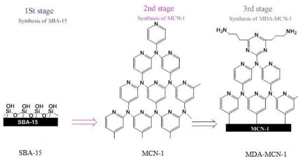
Fig. 1- Synthesis stages of MDA-MCN-1 from SBA-15 (hard template) to MDA-MCN-1.
