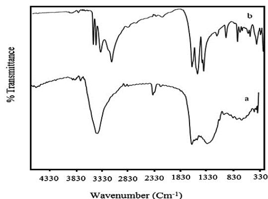
Fig. 4- FT-IR Spectra of MCN-1 (a) and MDA-MCN-1 (b) [21].
