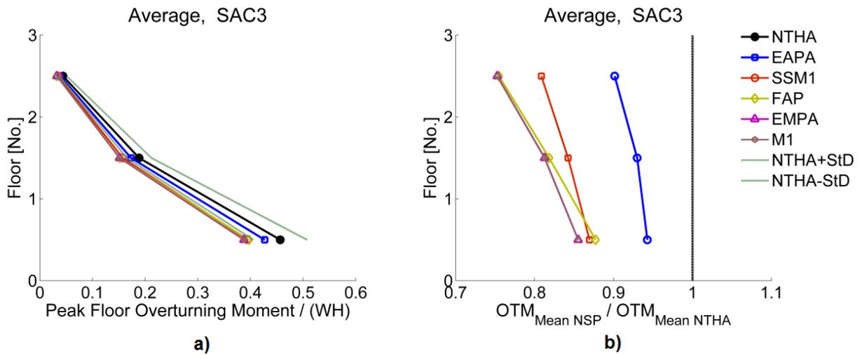
Fig. 6. a) The mean peak normalized floor overturning moment profiles and b) the mean peak floor overturning moment error profiles for SAC3
