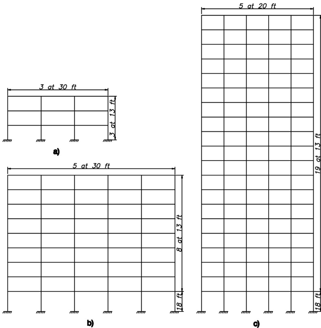
Fig. 3. Frame geometries of a) SAC3, b) SAC9, and c) SAC20 buildings
