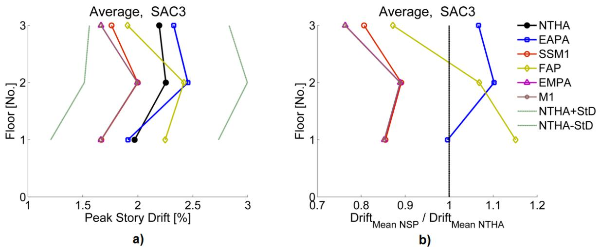
Fig. 4. a) The mean peak story drift profiles and b) the peak story drift error profiles for SAC3
