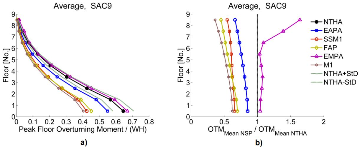
Fig. 10. a) The mean peak normalized floor overturning moment profiles and b) the peak floor overturning moment error profiles for SAC9
