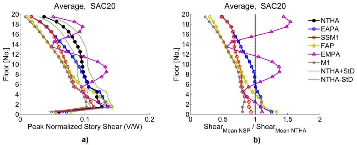
Fig. 13. a) The mean peak normalized story shear profiles and b) the mean peak story shear error profiles for SAC20
