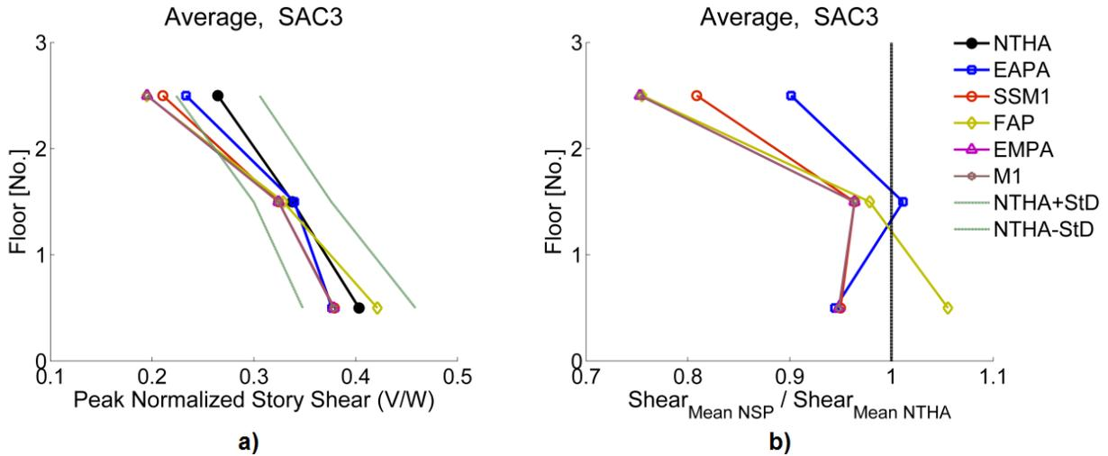
Fig. 5. a) The mean peak normalized story shear profiles and b) the mean peak story shear error profiles for SAC3
