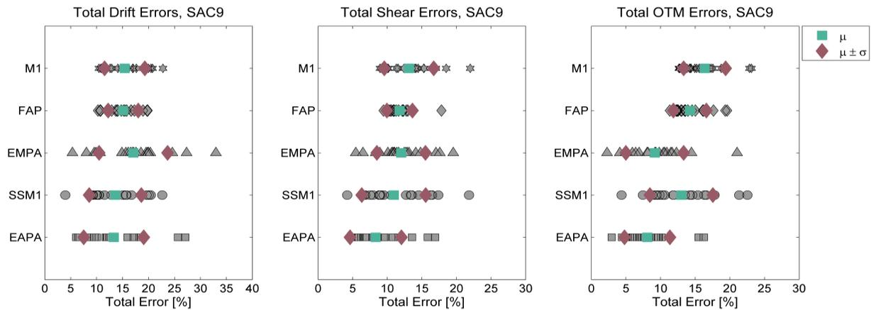
Fig. 11. Total errors for SAC9 in each NSP under all of the earthquake excitations along with the mean and mean +/- one standard deviation of them
