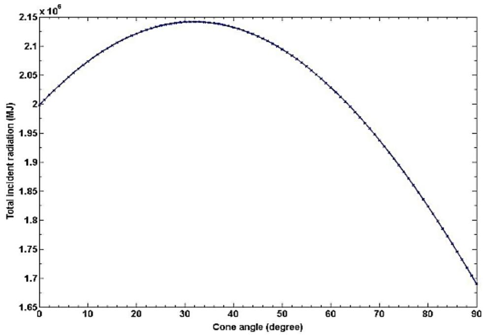
Fig. 6. Theoretical data for the total incident radiation on the conical collectors with respect to the cone angle (g).
