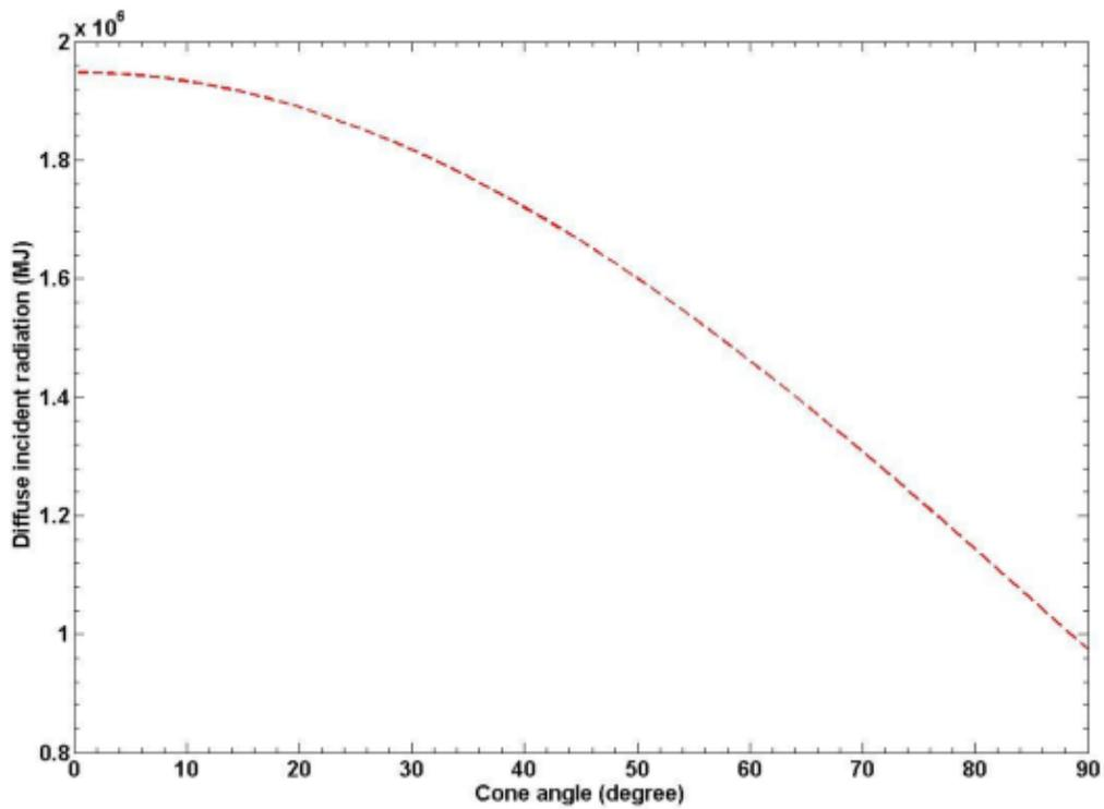
Fig. 7. Theoretical data for the diffuse radiation on the conical collectors with respect to the cone angle (g)
