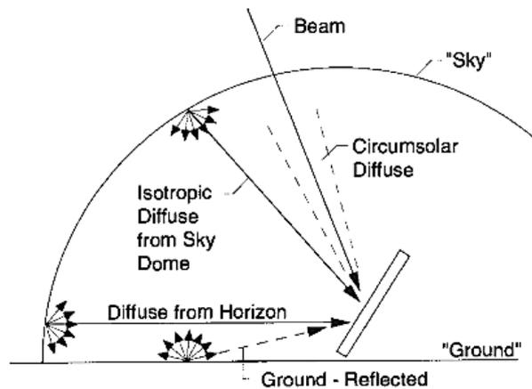
Fig. 2. Beam, diffuse, and ground-reflected radiation on a tilted surface [2]
