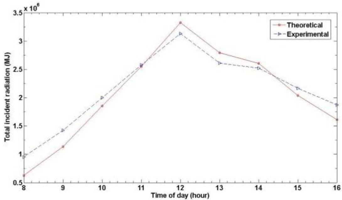
Fig. 8. Theoretical calculation and experimental measurement of the total incident radiation on the conical collector
