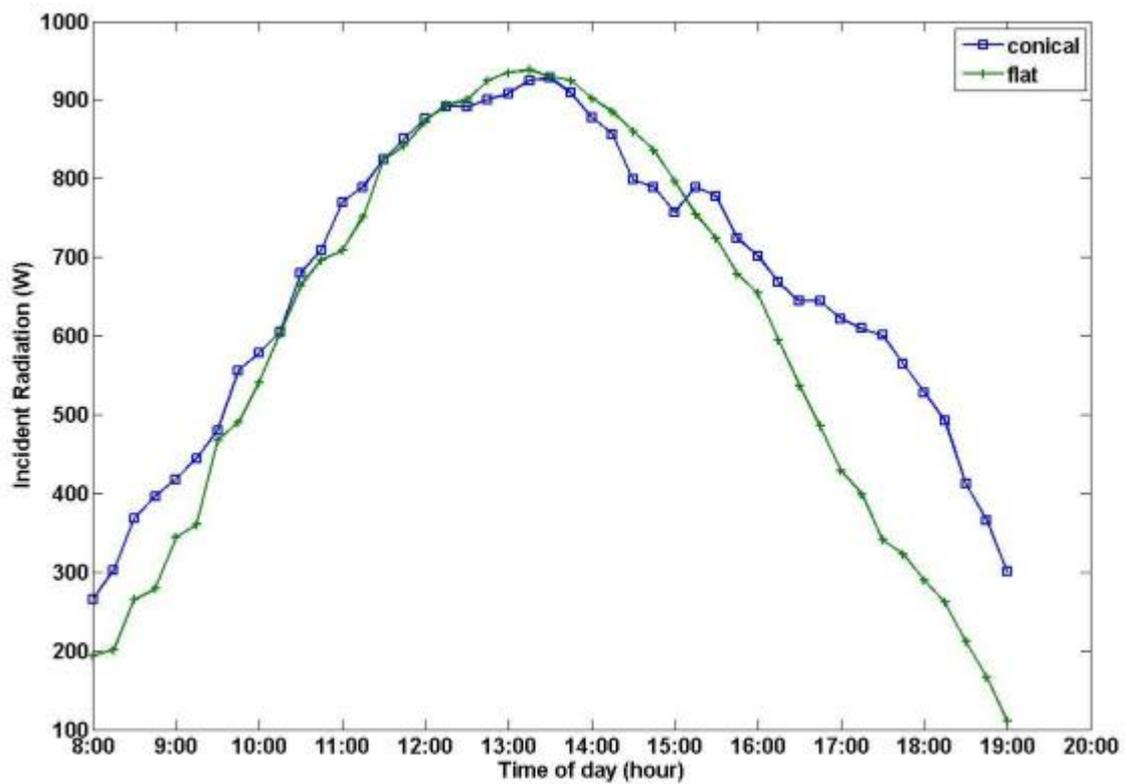
Fig. 9. Experimental data for the radiation on the flat and conical collectors (9.12.2014)
