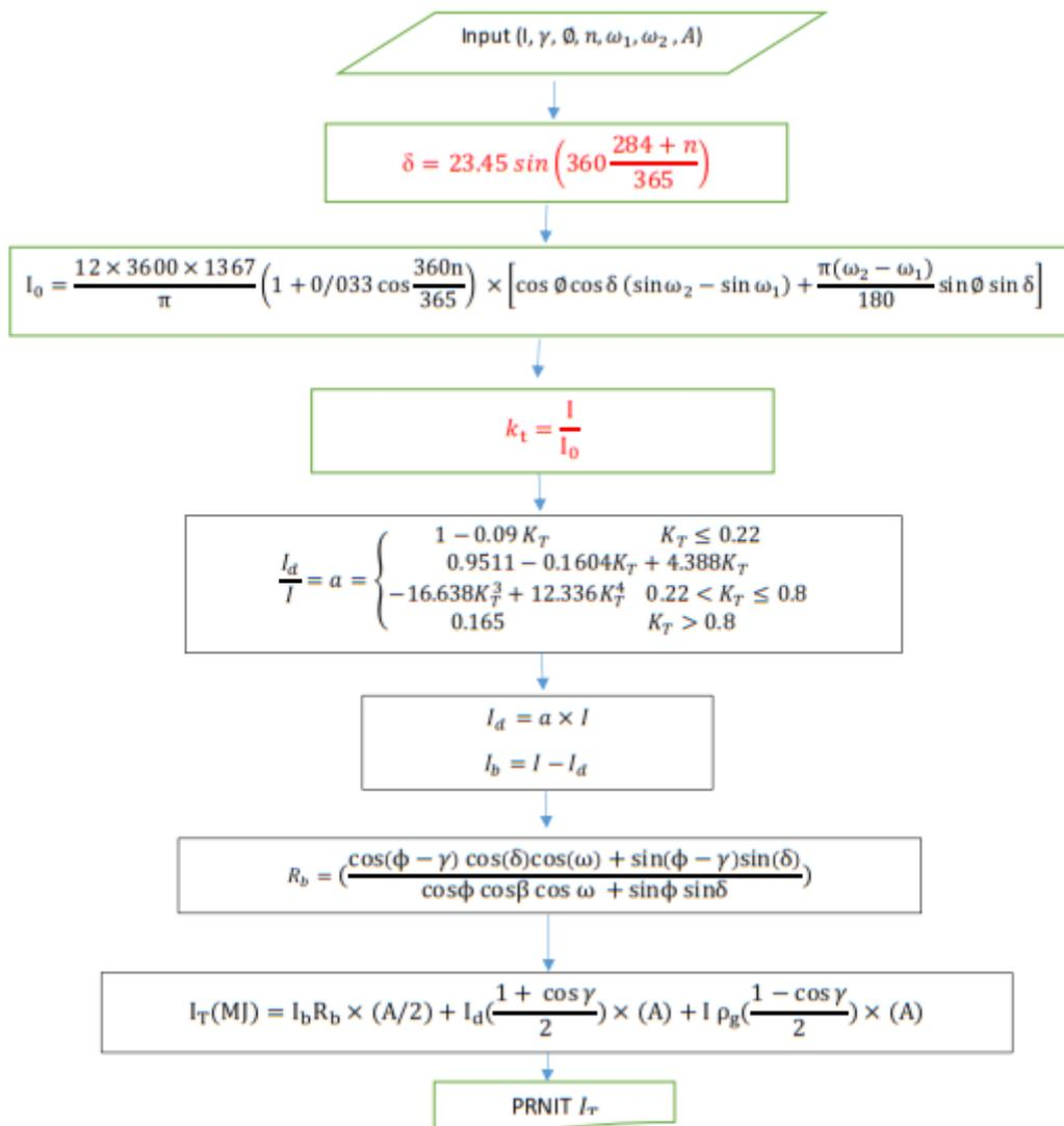
Fig. 3. Flowchart of step-by-step method to evaluate the total incident radiation on the conical solar collector
