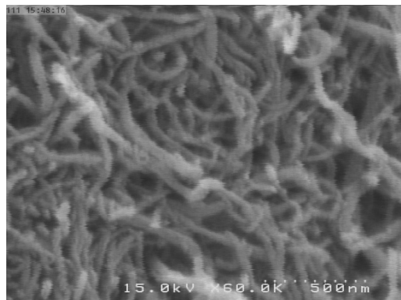
Fig. 4. Initial MWCNTs micro structure Scale: 500 nm
