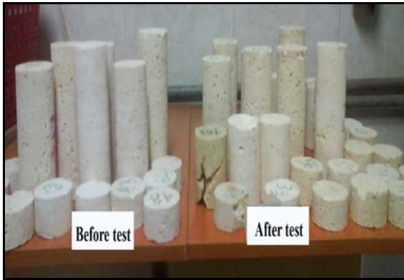
Figure 3. Limestone samples with various dimensions for freeze-thaw test (stage 1, and stage 5)
