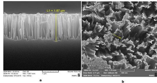
Fig. 3- (a) SEM image of Si NWs cross-section. (b) surface morphology of Si NWs
