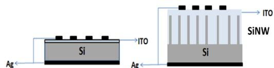
Fig. 1- Schematic diagram of Ag/ITO/Si Schottky solar cell, with and without Si NWs.
