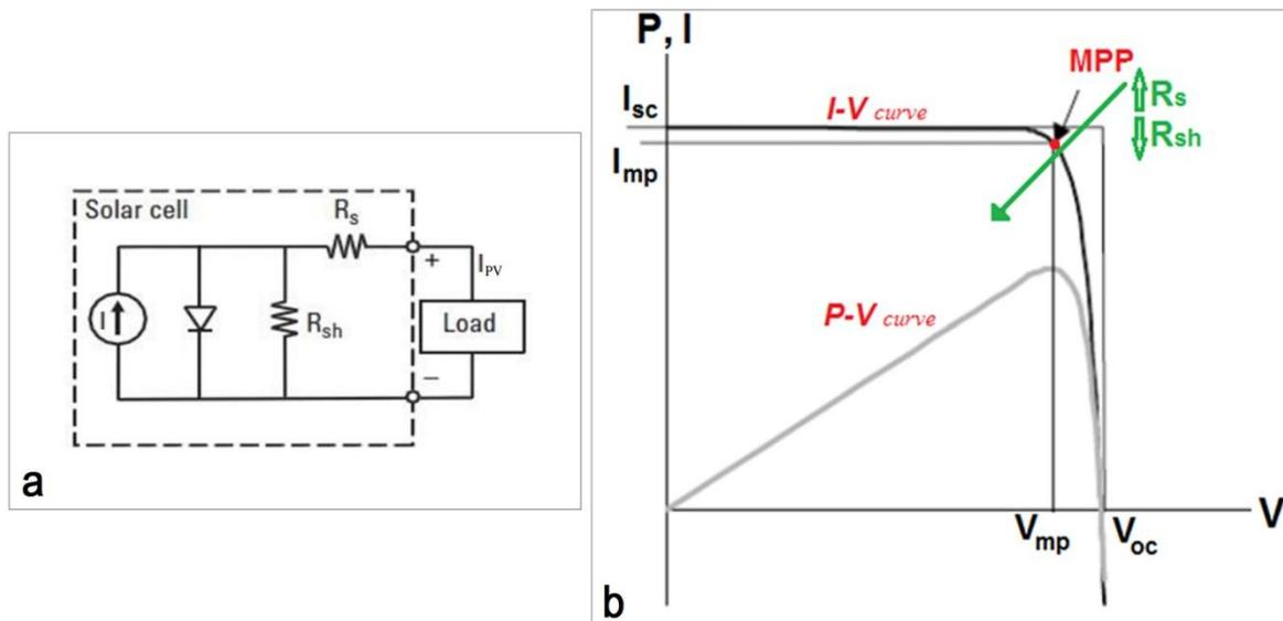
Fig. 2. Solar cell: a) equivalent circuit of a solar cell; b) I-V and P-V characteristic curves of a solar cell
