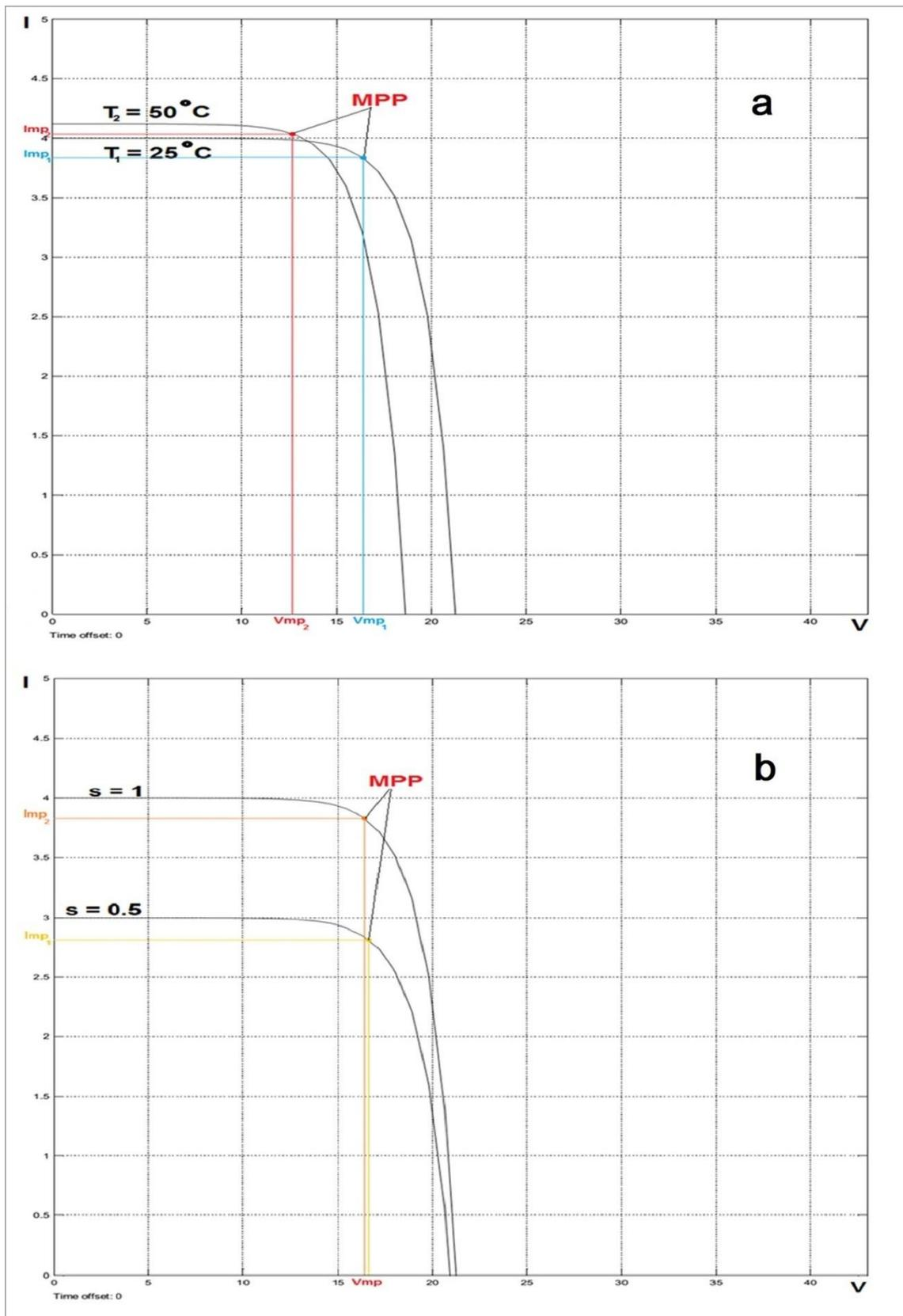
Fig. 4. Solar panel simulation: a) results at temperatures of 25°C and 50°C; b) results of simulated solar radiation at 500 and 1000 watts per square meter
