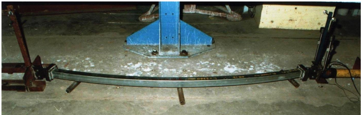
Fig. 6. Test set-up on the floor for long curved struts
