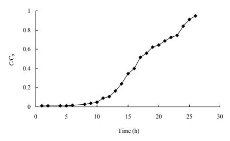
Fig. 6. Breakthrough curve for 2,4-D uptake from wastewater by SMSGW
