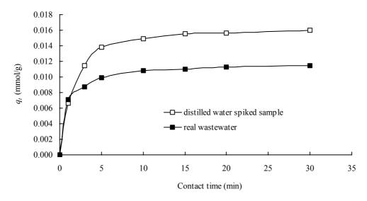
Fig. 2. Effect of contact time on 2,4-D uptake by SMSGW
