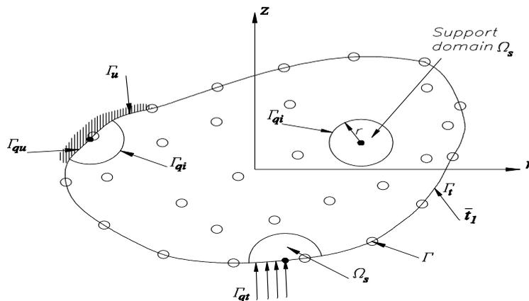
Fig. 2. Local domains used in the MLPG method
