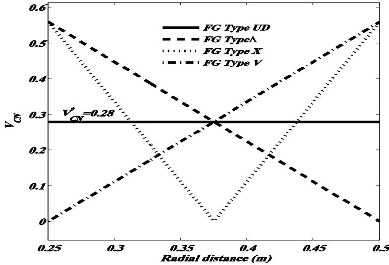
Fig. 1. Four types of variation of nanotube volume fraction ( $V_{CN}$ ) along the radial direction
