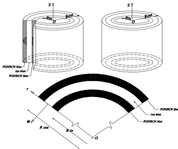
Fig. 4. Cylindrically layered structure with three layers
