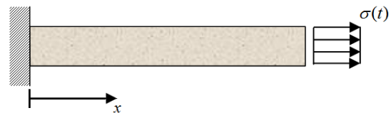
Fig. 8. The first example. A sample rod excited by an end stress field
