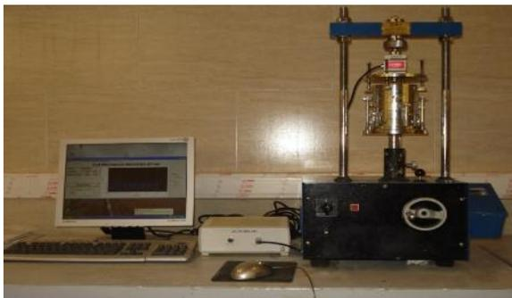
Figure 1. Pull-out adhesion testing device
