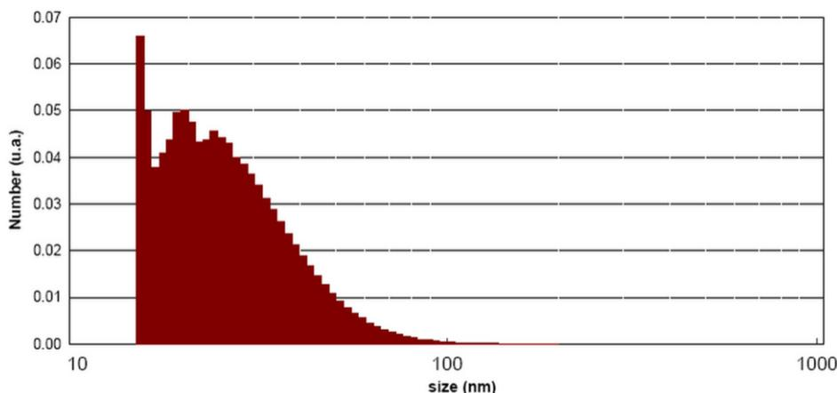
Fig. 7. Size distribution of the CuO nanoparticles
