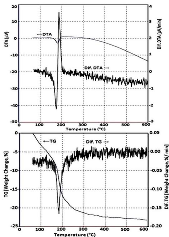
Fig. 3. DTA and TGA curves of as-prepared  $\text{Cu}(\text{OH})_2$
