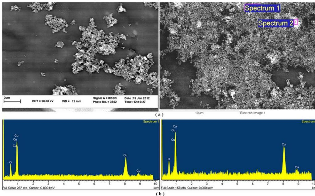
Fig. 5. a) SEM micrographs and b) EDS patterns of CuO powders
