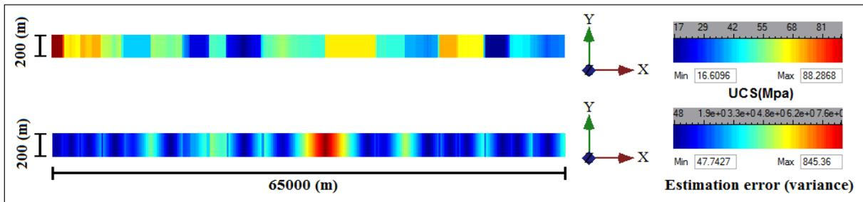
Fig. 6. Distribution of estimated UCS and variance of estimation error along the tunnel axis
