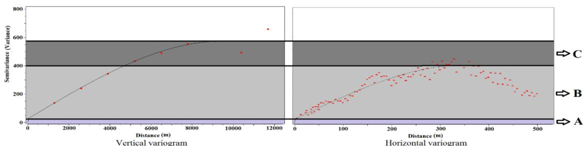
**Fig. 5. general structures of variance: a) first structure (nugget effect), b) second structure (geometric anisotropy), and c) third structure (regional anisotropy)**
