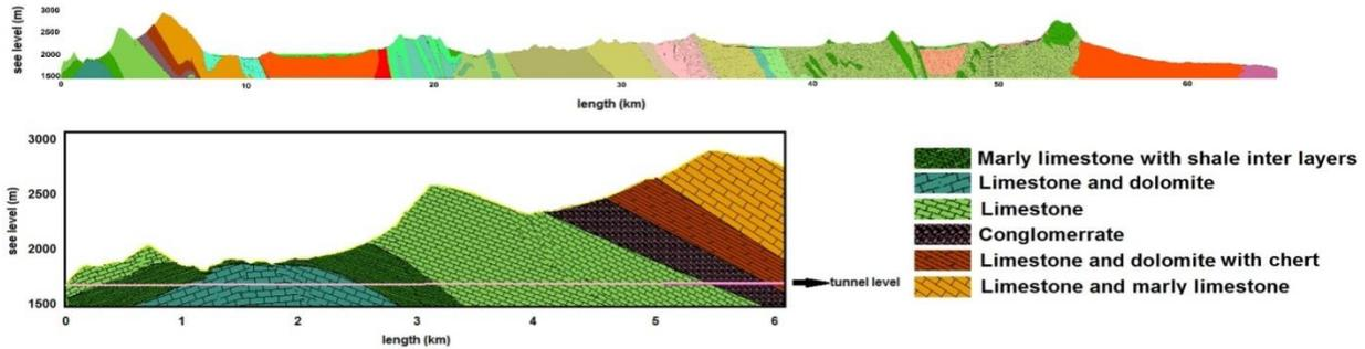
Fig. 1. geological profile of the tunnel route [17]
