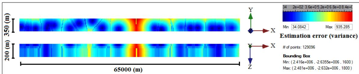
Fig. 8. Distribution of the variance of estimation error in the vicinity of exploratory boreholes
