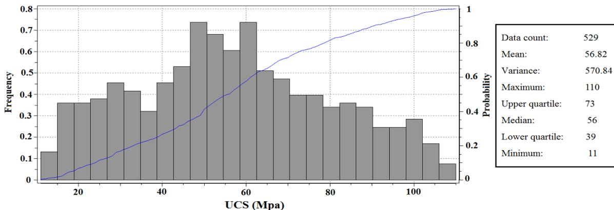
Fig. 3. Histogram of values of UCS obtained from laboratory tests
