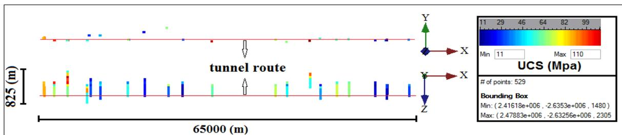
Fig. 2. distribution of reliable UCS test results in boreholes
