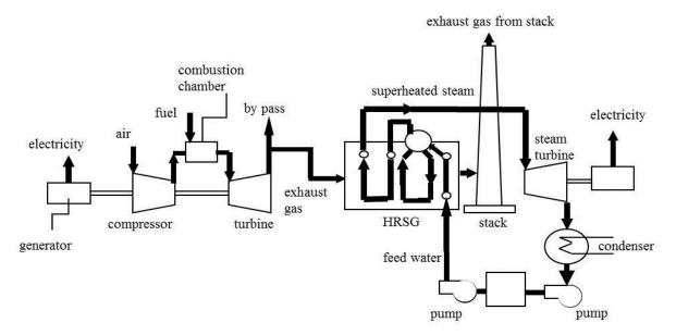
Fig. 1. Schematic view of a combined cycle
