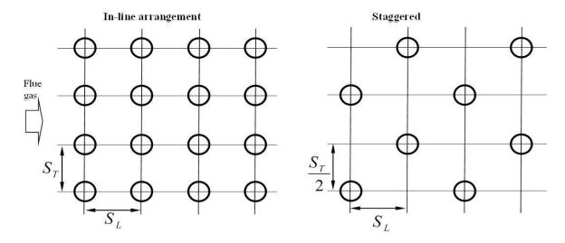
Fig. 3. Tube arrangements in HRSGs
