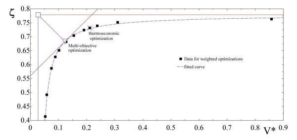
Fig. 5. Variations of normalized irreversibility and exergetic efficiency versus normalized equivalent volume
