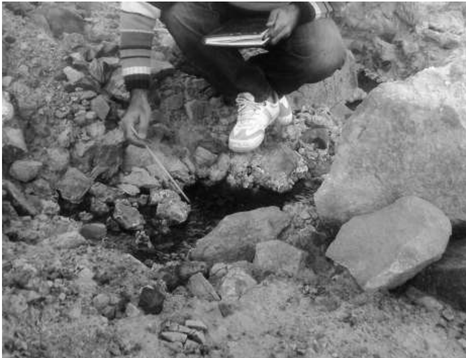
Figure 2. Measuring the temperature of PLS in Sarcheshmeh heap No. 1.
