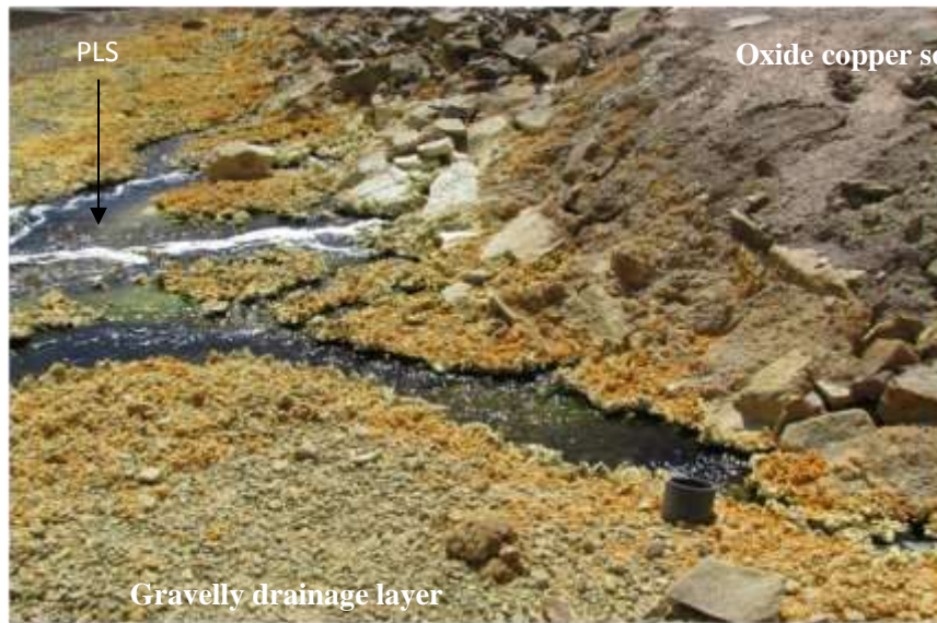
Figure 1. Drainage of PLS through a gravelly drainage system (Sarcheshmeh copper heap leaching structure No.1).
