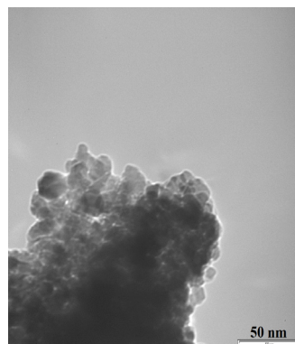
Fig. 10- TEM image of alumina after solving metallic nickel in nitric acid.
