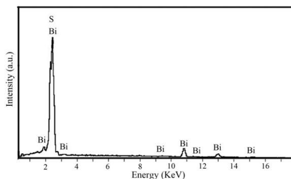
**Fig. 2.** EDS spectrum of the as synthesized Bi<sub>2</sub>S<sub>3</sub> nanorods at 50 W for 30 min (sample 3).
