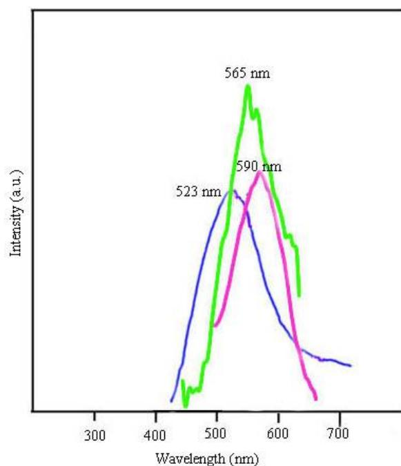
**Fig. 4.** PL spectrum of the as synthesized  $\text{Bi}_2\text{S}_3$  nanorods (a) sample 2 (b) sample 3 (c) sample 8.
