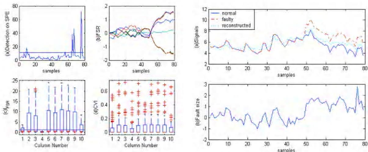
Fig. 13. (Left) Sensor fault detection and identification of DO sensor bias (a) SPE plot, (b) FSR, (c)  $I_{FSR}$ , (d) CVI, (Right) Sensor reconstruction of DO sensor bias (a) normal, faulty and reconstructed signals, (b) fault size
