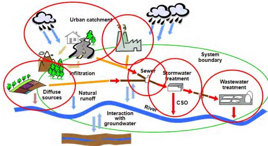
Fig. 1. System components of urban water cycle
