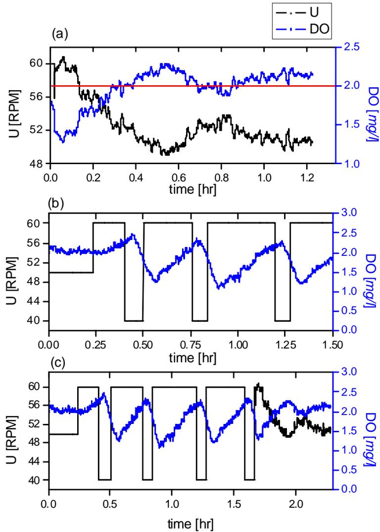
**Fig. 8. Experimental results of different process identification methods of DO concentration and speed of the surface aerator in a full-scale WWTP. (a) Set-point change of PID controller, (b) relay feedback, and (c) relay-plus proportional controller**
