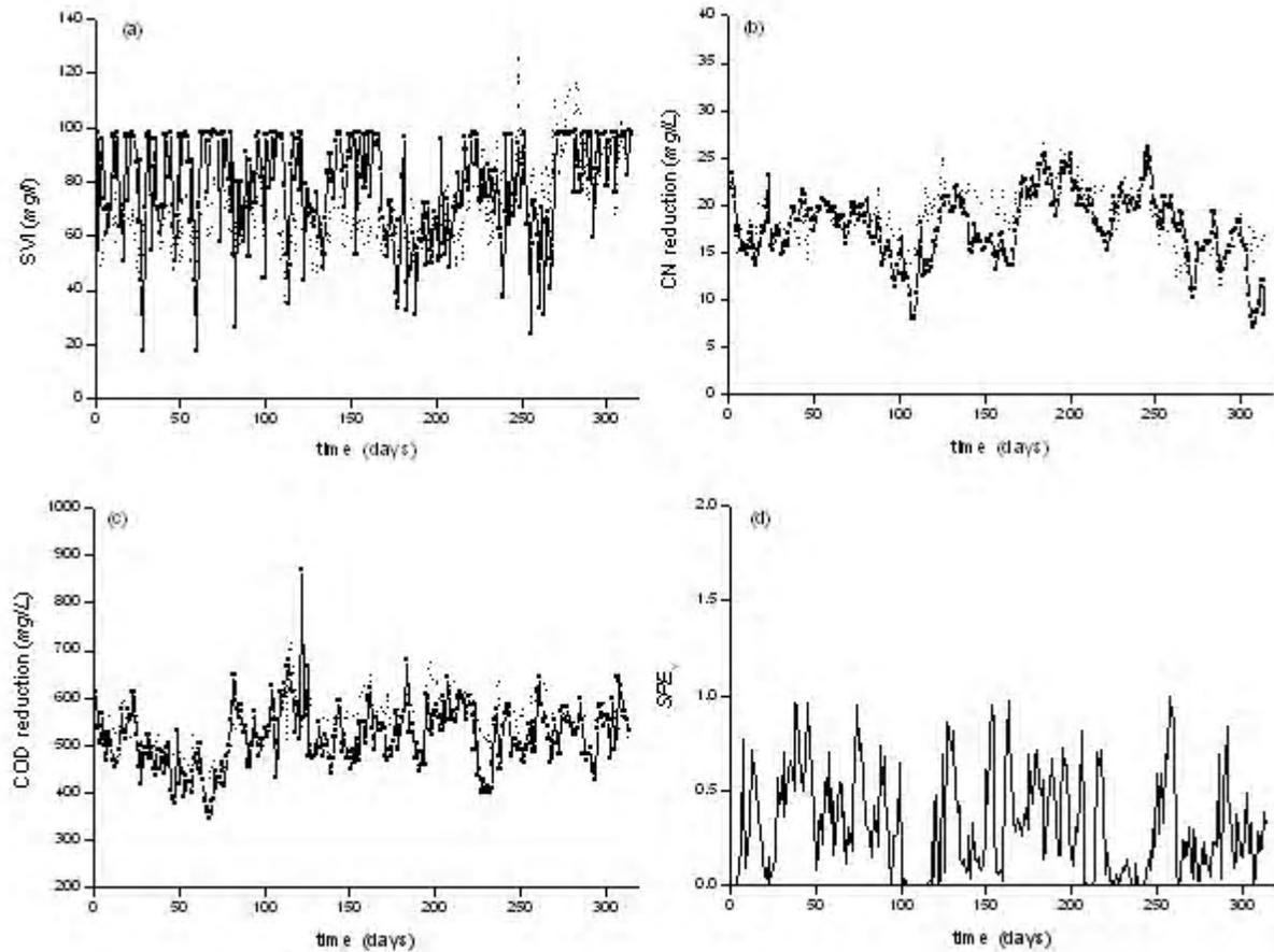
**Fig. 7. Prediction results of the PLS model with real  $Y$  value (solid line with squares) and predicted value (dotted line), (a) SVI, (b) reduction of CN, (c) reduction of COD, (d) squared residual error of  $Y$  variables ( $SPE_Y$ )**
