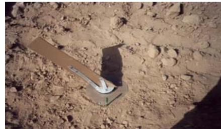
Fig. 3. Near-surface sampler used to measure the sediment mass flux close to the eroding surface
