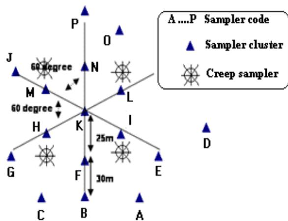
Fig. 4. Schematic layout of field site instrumentation
