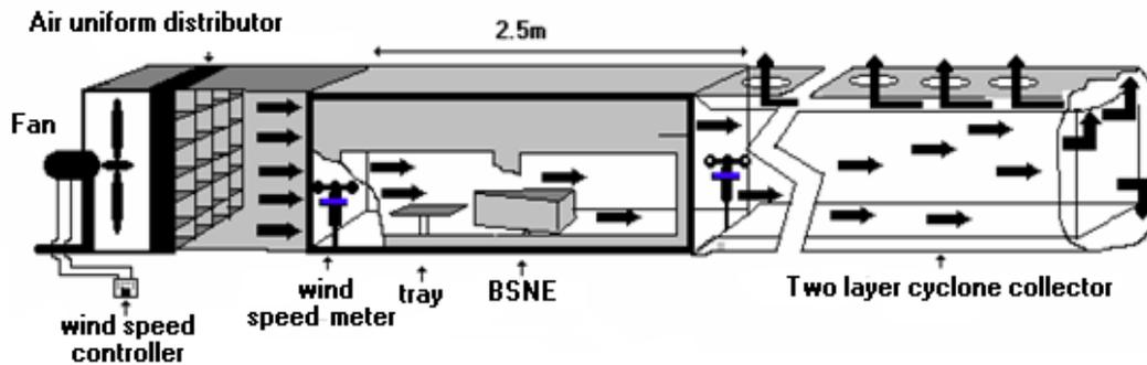
Fig. 5. Test procedure for determining sampling efficiency of assembled sampler
