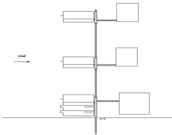
Fig. 2. BSNE (Big Spring Number Eight) sampling cluster used to measure sediment mass flux at various heights above a wind-eroding surface (schematic and in field)
