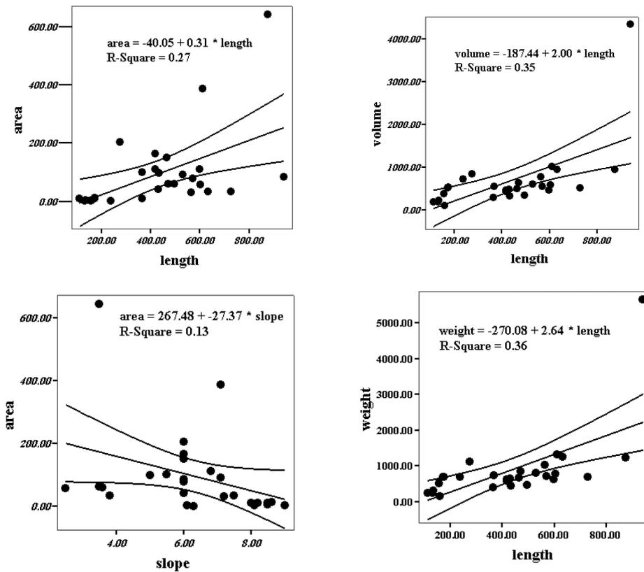
Fig. 6. Relationship between gully physical properties (Volume in cubic meter, length in meter, area in hectare, weight in ton and slope in percentage)
