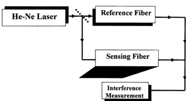
**Figure 1.** The block diagram of a Mach-Zehnder interferometer that can be used for temperature sensing.
