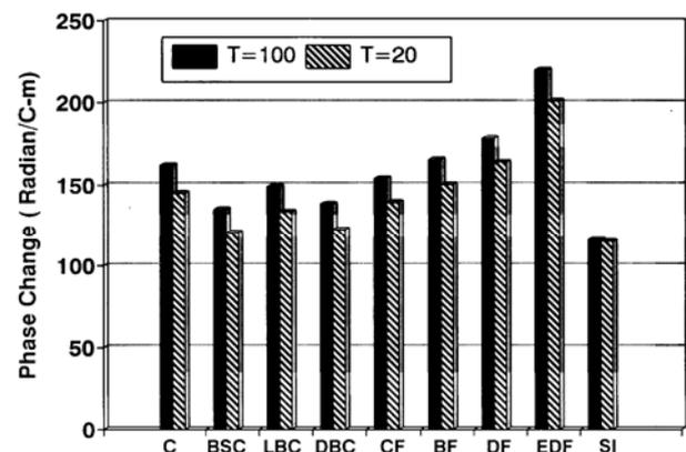
Figure 3. The phase changes for different optical glasses for two temperatures.
