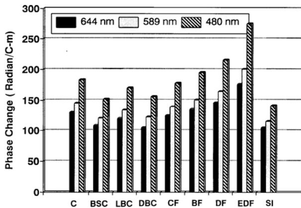
Figure 4. Shows the phase variation as function of source wavelength for different optical glasses.
