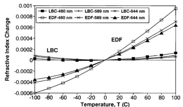
Figure 2. Variation of the index of refraction with respect to temperature for different wavelengths.
