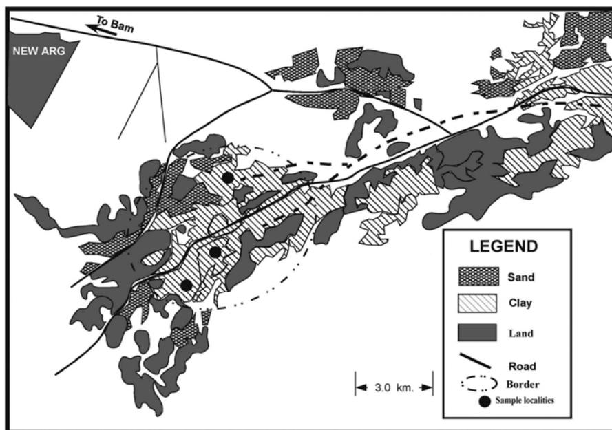
Figure 2. Generalized geological map of Nazem-Abad area (from satellite photo).
