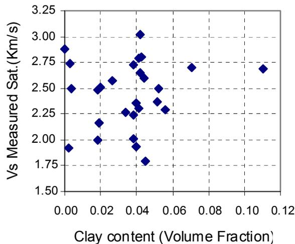
Figure 8 - Effect of clay content on shear wave velocity.
