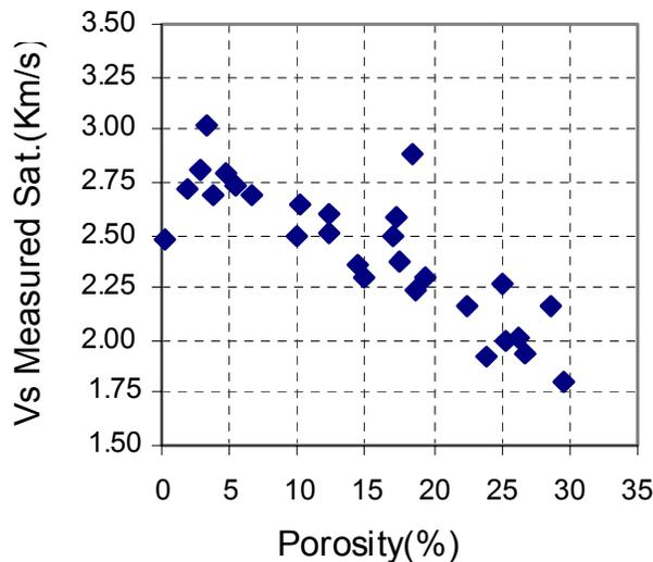
Figure 9 - Effect of porosity on shear wave velocity.
