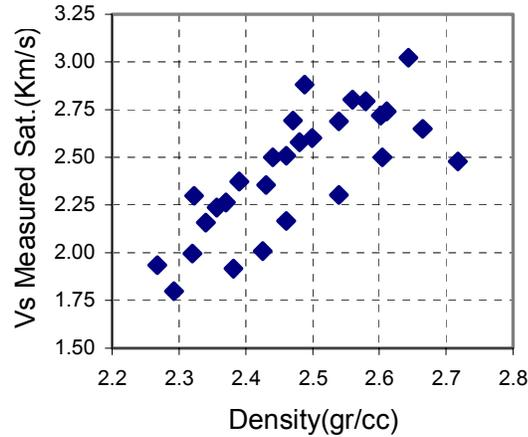
**Figure 10 -Effect of bulk density on shear wave velocity.**
