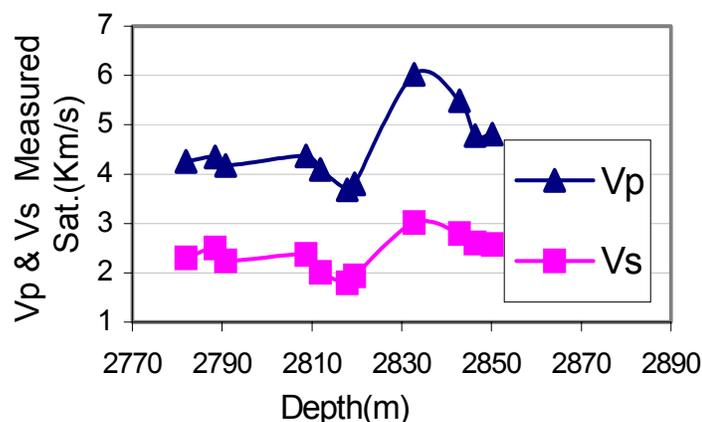
Figure 4 – A comparison between  $V_p$  and  $V_s$  in well 3, showing a good match.
