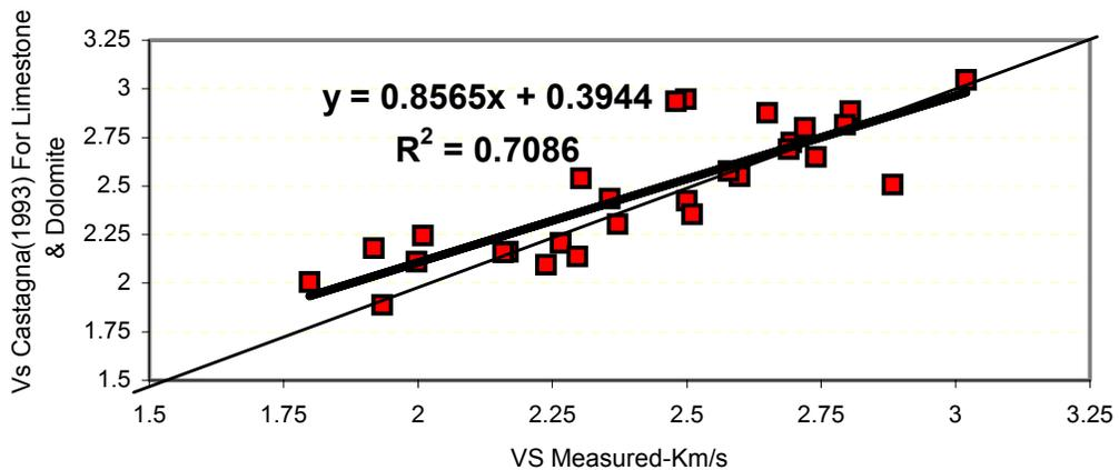
**Figure 6 - Plot of calculated  $V_s$  from Castagna et al., (1993) equation versus measured  $V_s$  at 30Mpa effective stress and 100% water-saturated condition.**
