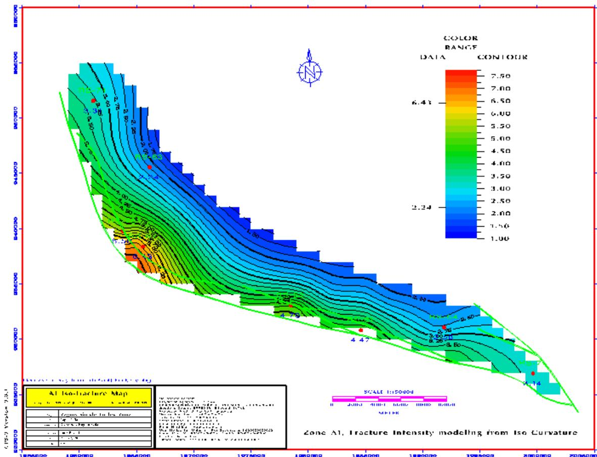
Figure 9. Iso-Fracture map of Rag-e Sefid structure
