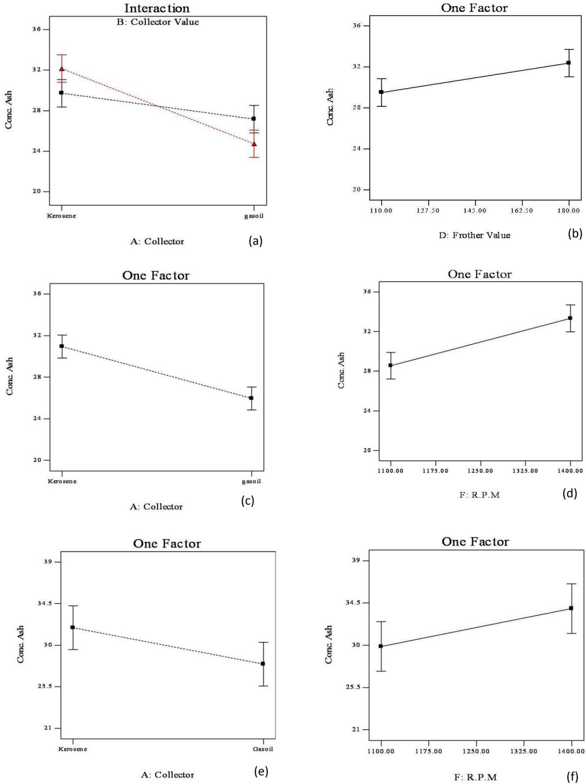
**Figure 6: Effect of effective parameters on concentrate ash: A) non ground sample, B) ground sample. Choosing gasoline for both samples causes a decrease in ash content. The increase of rpm increases the product ash and less amount of frother should be used for non ground sample.**
