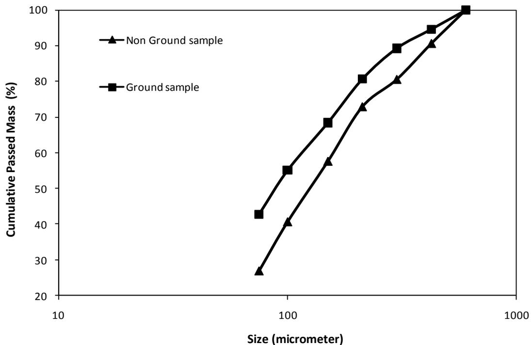
**Figure 1: Size distribution of ground and non ground samples, used in flotation process**
