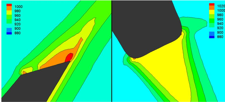
**Fig.3.** Entropy generation at the trailing edge of the rotor (left) and the stator (right).
