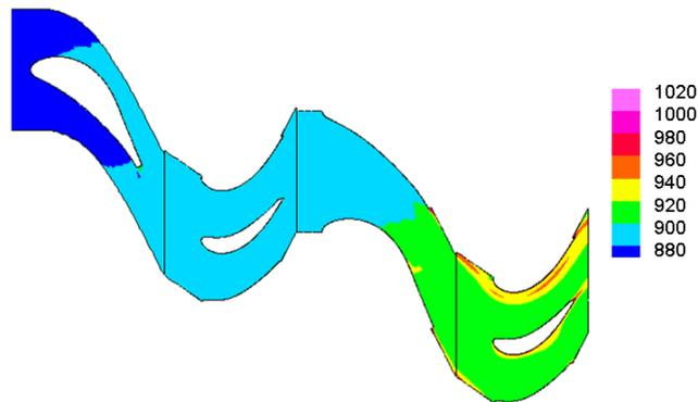
**Fig.4.** Entropy distribution for the clocking position S1.
