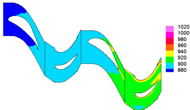
**Fig.6.** Entropy distribution for the clocking position S3.
