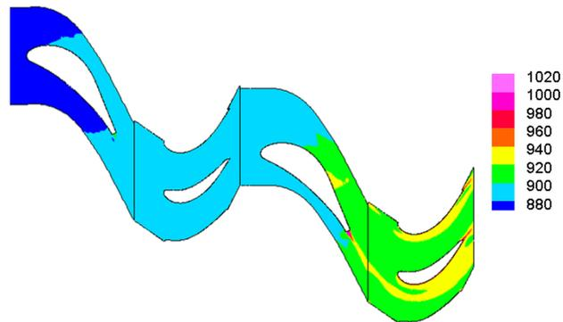
**Fig.5.** Entropy distribution for the clocking position S2.
