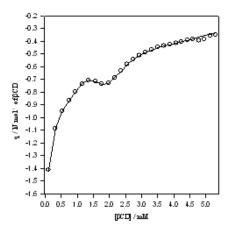
**Figure 1.** Comparison between the experimental heats, q, (O), for lysozyme+ $\beta$ CD interaction and calculated data (lines) via Eq. 1. [ $\beta$ CD] are concentrations of  $\beta$ CD solutions in mM at pH 12.
