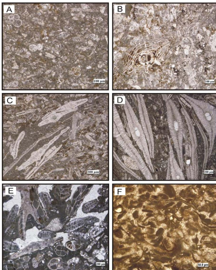
**Fig. 3: Microfacies types of Asmari Formation A- MF1: Bioclast planktonic foraminifera wackestone-packstone B- MF2: Lepidocyclinidae nummulitidae planktonic foraminifera bioclast wackestone-packstone C- MF3: Nummulitidae bioclast wackestone-packstone D- MF4: Bioclast lepidocyclinidae nummulitidae packstone E- MF5: Lepidocyclinidae nummulitidae bryozoa packstone-grainstone F- MF6: Bioclast peloidal grainstone (XPL).**
