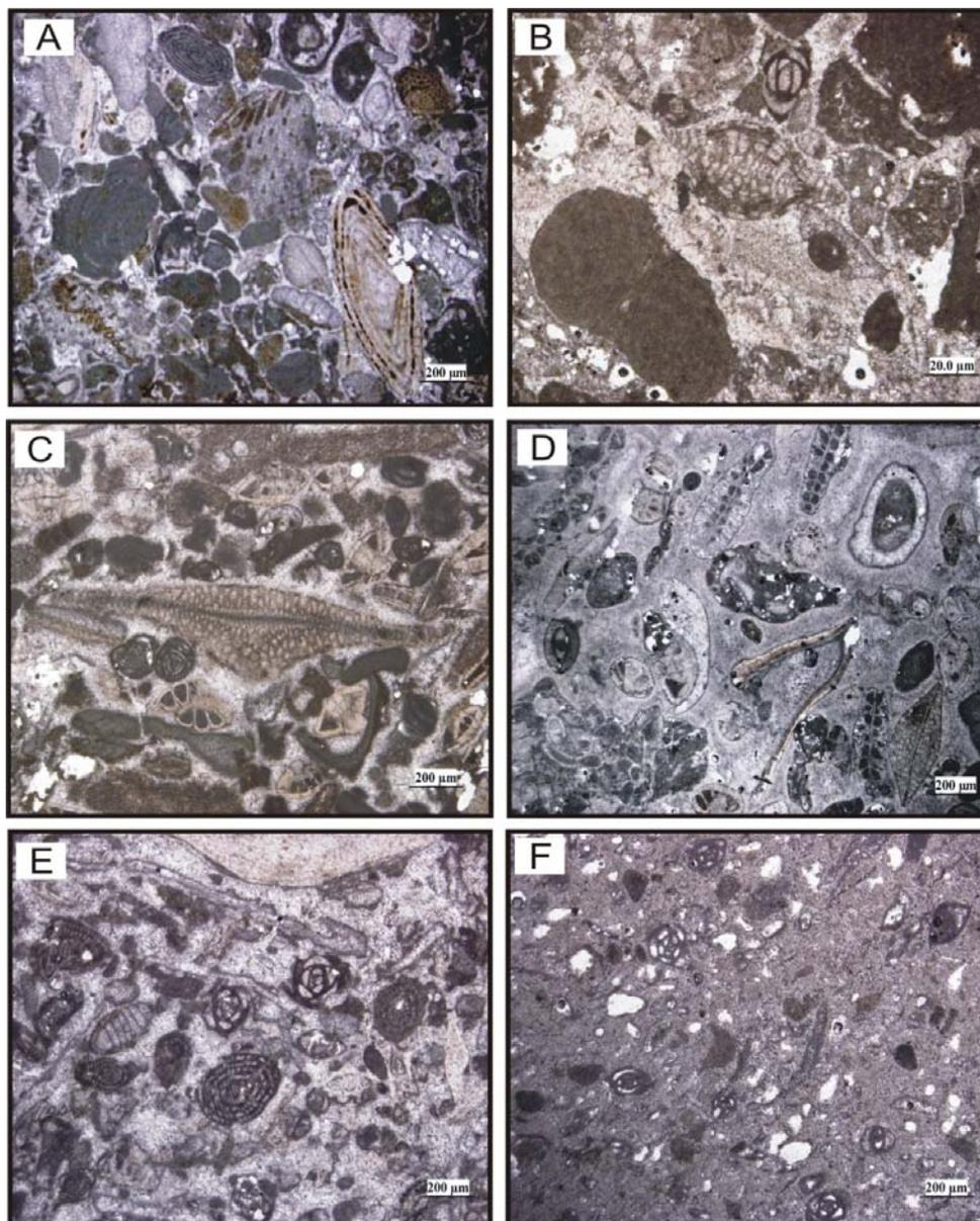
**Fig. 4:** Microfacies types of Asmari Formation A- MF7-a: Benthic foraminifera (perforate and imperforate) bioclast wackestone-packstone-grainstone B- MF7-b: *Norotalia* benthic foraminifera bioclast packstone C- (MF7-c): Benthic foraminifera corallinacea packstone D- MF7- d: Benthic foraminifera bioclast bryozoa packstone E- MF8: Imperforate foraminifera bioclast wackestone-packstone-grainstone F- MF9: Miliolid bioclast wackestone (XPL).
