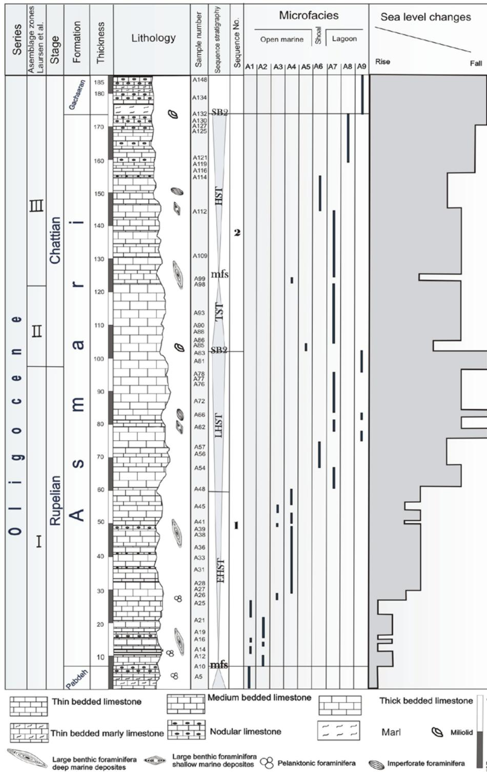
**Fig. 6: Vertical microfacies distribution and sequences of the Asmari Formation at Firozabad section, Zagros. TST: Transgressive Systems Tract; HST: Highstand Systems Tract; MFS: maximum flooding surface; SB2: Sequence boundary type 2**
