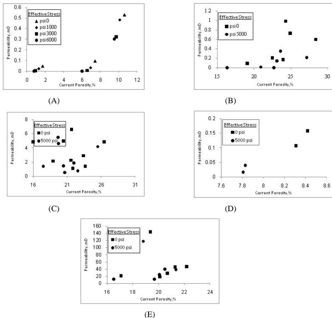
**Figure 5: Permeability vs. current porosity at different effective stress levels for different rock types (A: crystalline limestone, B: separated vuggy pores limestone, C: touching vuggy pores limestone, D: mud- dominated dolomite and E: grain-dominated dolomite.)**
