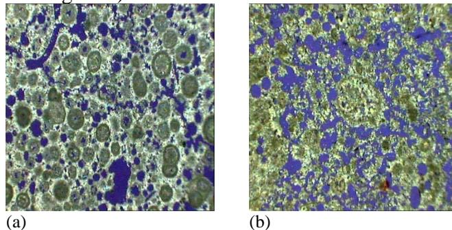
**Figure 1: Limestone thin sections; (a) separated vuggy pores limestone and (b) well-connected vuggy pores limestone.**
