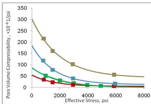
**Figure 3: An example of compressibility-stress curves for 4 samples of crystalline limestone, dashed lines are theoretical fitted correlation and cubic marks represent experimental data.**
