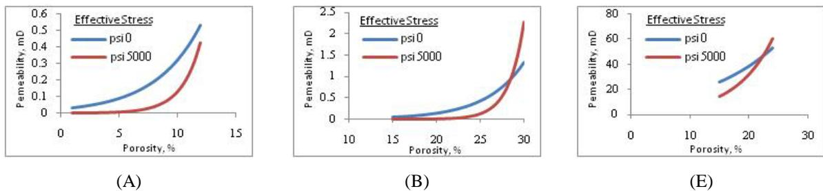
Figure 6: Exponential correlation between permeability and porosity (A: crystalline limestone, B: separated vuggy pores limestone, and E: grain-dominated dolomite.)
