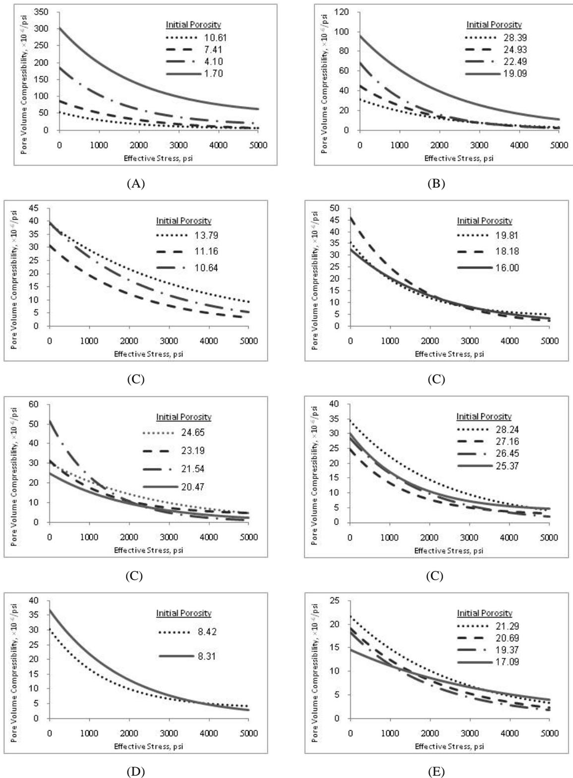
Figure 4- Relationship between pore volume compressibility and effective stress for different rock types at different initial porosity (A: crystalline limestone, B: separated vuggy pores limestone, C: touching vuggy pores limestone, D: mud-dominated dolomite and E: grain-dominated dolomite.)
