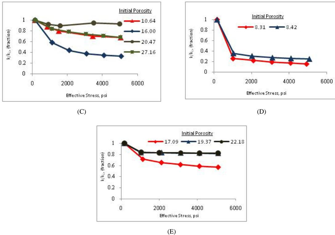
Figure 7: Permeability fraction ( $k/k_0$ ) vs. effective stress at different initial porosity for different rock types (A: crystalline limestone, B: separated vuggy pores limestone, C: touching vuggy pores limestone, D: mud-dominated dolomite and E: grain-dominated dolomite.)
