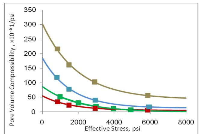
**Figure 3: An example of compressibility-stress curves for 4 samples of crystalline limestone, dashed lines are theoretical fitted correlation and cubic marks represent experimental data.**
