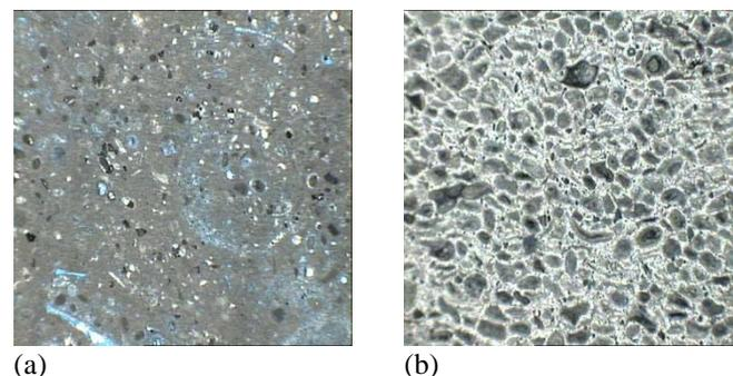
**Figure 2- Dolomite thin sections; (a) mud-dominated dolomite and (b) grain-dominated dolomite.**
