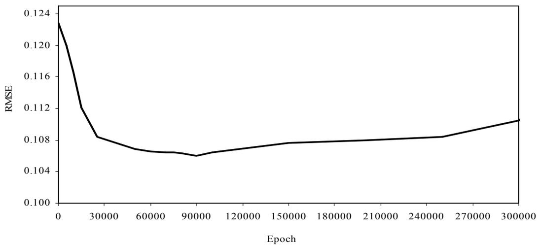
Figure 11. RMS error graph for MLP network with sigmoid function for all layers.
