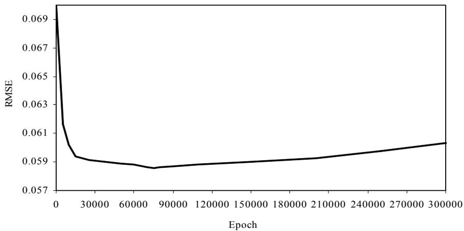
Fig. 8. RMSE graph for MLP network with TANH threshold function for the first and second hidden layers and linear for the third and output layers
