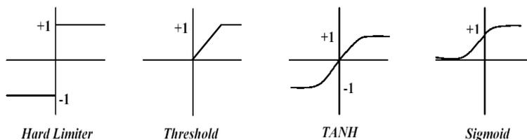
Fig. 3. The most important functions for activation of neurons (3)
