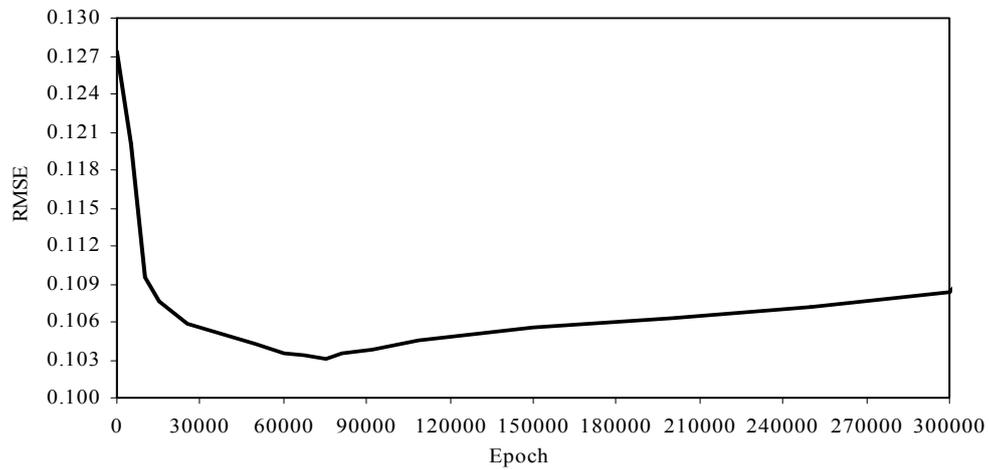
Fig. 10. RMS error graph for MLP network with sigmoid threshold function for the first and second hidden layers and linear for the third and output layers
