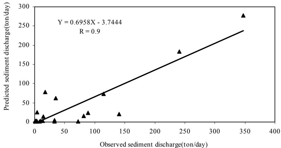
Fig. 5. MLP network test with TANH threshold function
