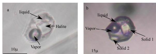
**Figure 4.** Photomicrograph of fluid inclusions in skarn calcite from the Sangan deposit. (a) Three phase fluid inclusion, (b) Four phase fluid inclusion.
