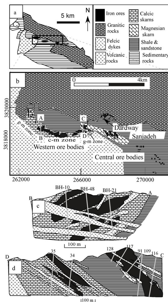
**Figure 2.** Simplified geological maps (a and b) showing distribution of the iron ores in the Sangan deposit. c) a N-S cross section from g-m zone, d) a N-S cross section from magnesian zone ( north side) and g-m zone (south side). g-m = garnet-magnetite and c-m = carbonate-magnetite, BH = borehole.
