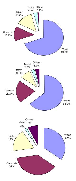
Fig. 4. Composition of construction waste at sites A, B and C
