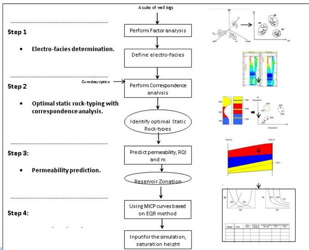
Figure1: Flow diagram summarizing the integration of data suite into dynamic rock-type characterization
