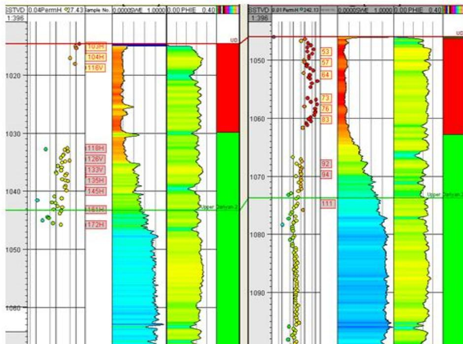
**Figure6: A well section of availability MICP samples with well logs (porosity and Sw)**
