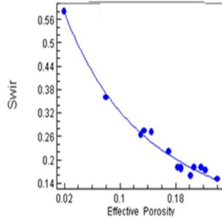
**Figure8: Correlation of irreducible water saturation versus effective porosity based on pay zone**
