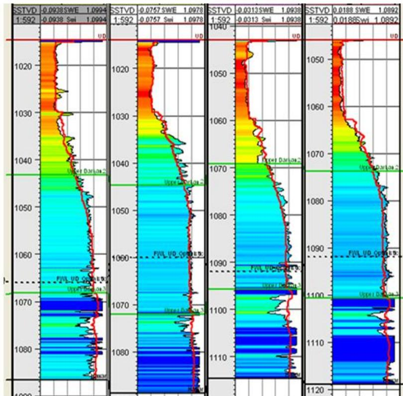
**Figure9: Comparison of water saturation of measured versus calculated**
