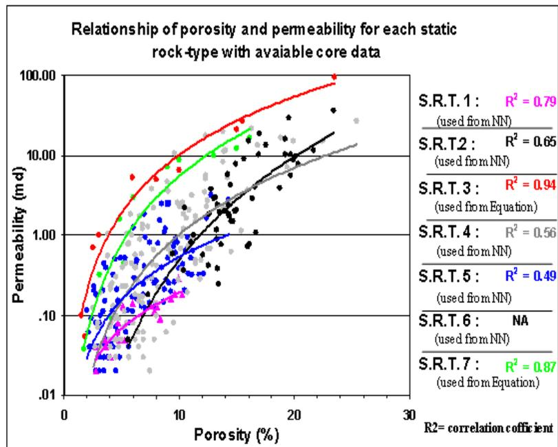
Figure3: Relationship of porosity and permeability for each SRT in well no.
