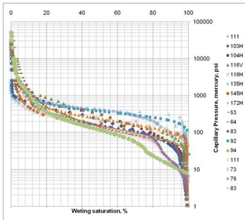
Figure 4: Mercury injection capillary pressure for available data
