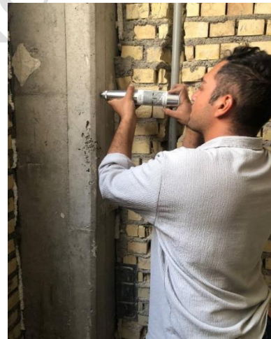
Fig. 4. Performing the Schmidt hammer test on the column
