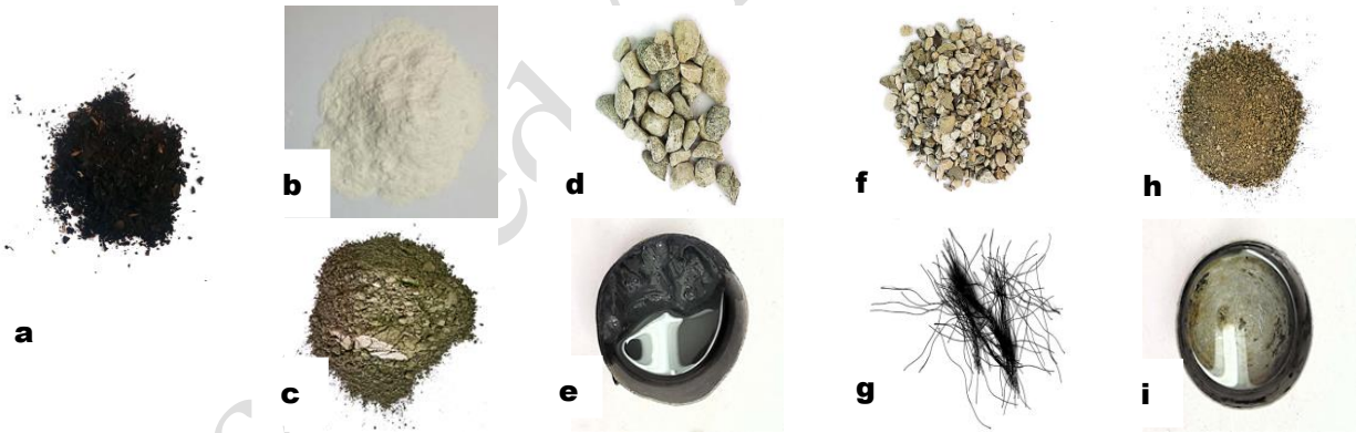
Fig. 2. Components used in the formulation of ultra-high-strength concrete, with and without basalt fibers: a) Silica sand, b) Quartz powder, c) Type II Portland cement, d) Almond sand, e) Nano silica gel, f) Pea sand, g) Basalt fibers, h) Sand, i) Potable water
