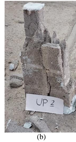
Fig 6. Performance of the unconfined prisms (UPs) under axial compression; a) Compression stress-strain curve, b) Typical failure pattern
