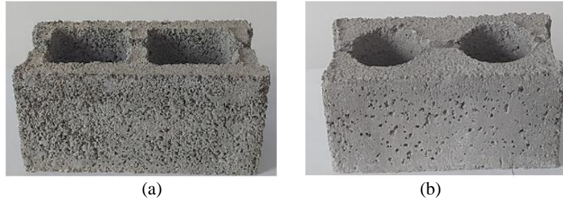
Fig 2. Typical half-scale concrete masonry blocks (all dimensions in mm); a) Conventional stretcher unit, b) Self-reinforced (SR) unit
