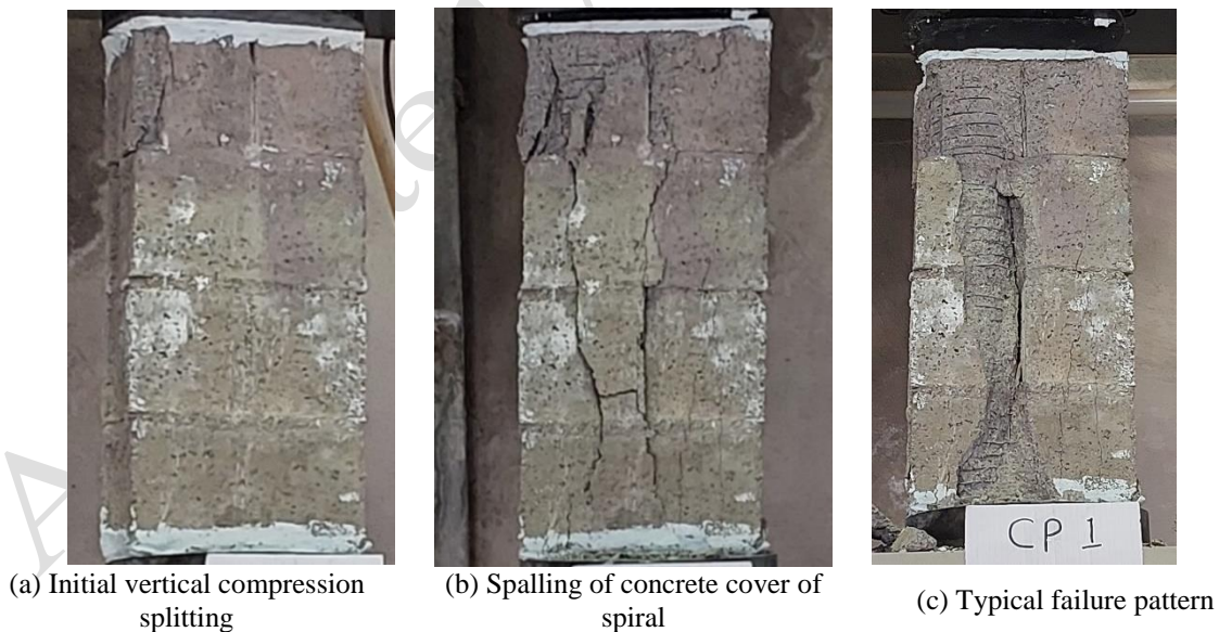
Fig 7. Damage initiation and failure pattern of a typical Confined prism (CPs)
