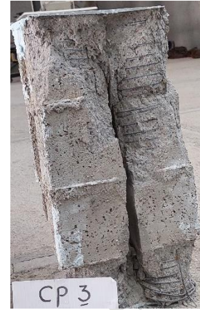
Fig 8. Performance of the confined prisms (CPs) under axial compression; a) Compression stress-strain curve, b) Typical failure pattern
