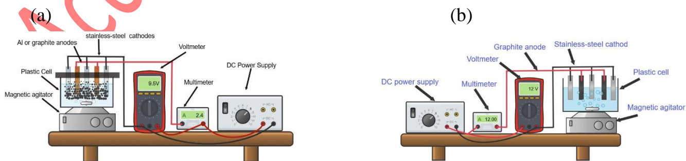
Figure 1: (a) Diagram of the sequential EC &EO process, (b) Diagram of the sequential EO process
