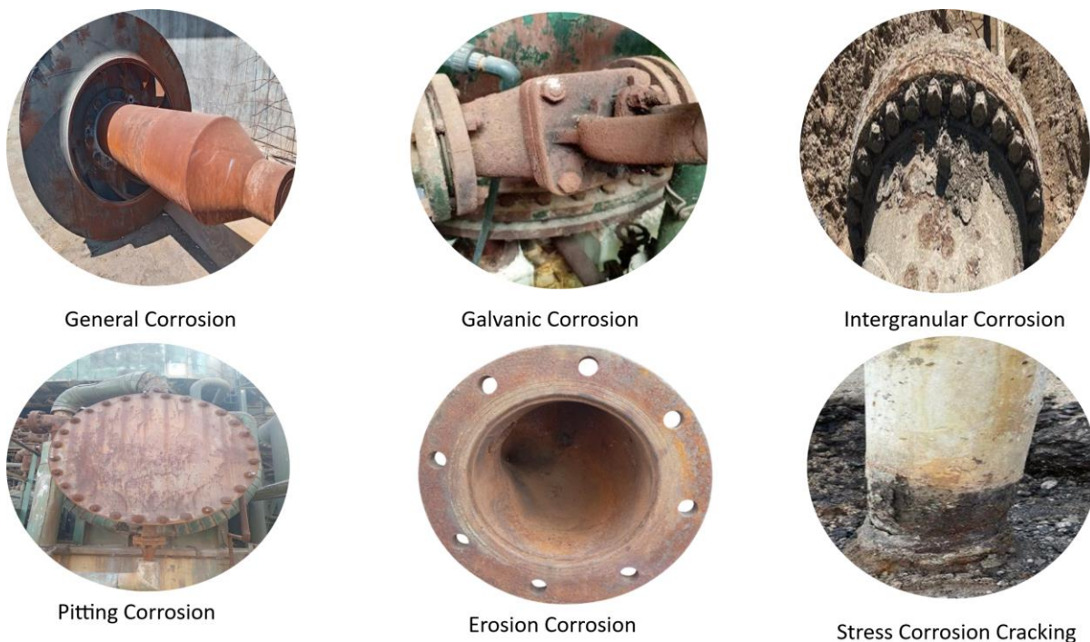
Fig. 7. Different corrosion patterns in carbon steels manufactured parts as observed at the thermal power station and refinery of Al-Dora-Baghdad, Iraq
