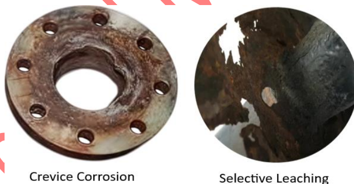
Fig. 8. Crevice corrosion and selective leaching [98,100]
