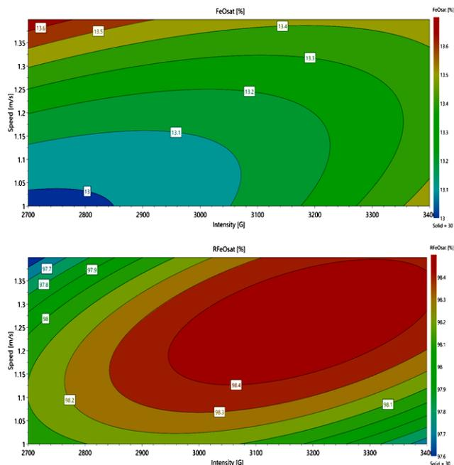
Fig. 7. Contour plots related to the grade response and recovery of iron oxide from the satmagan.
