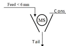
Fig. 3. Final flowsheet. Feed finer than 6 mm was separated by a wet magnetic separator.
