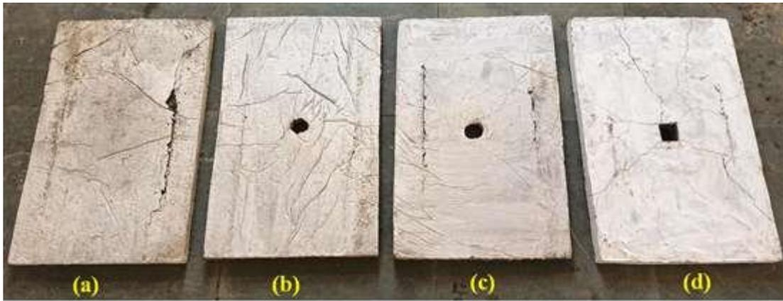
Figure 6. Crack pattern in RCC slab: without (a) opening and with (b) hexagonal, (c) circular and (d) square opening.
