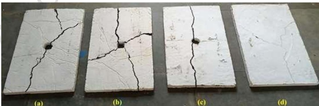
Figure 5. Crack pattern in PCC slab with: (a) hexagonal, (b) square, (c) circular and (d) slab without any opening.
