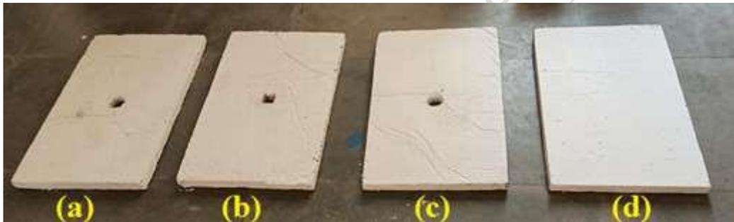
Figure 2. Slab specimens with hole: (a) hexagonal, (b) square, (c) circular and (d) slab without any hole.
