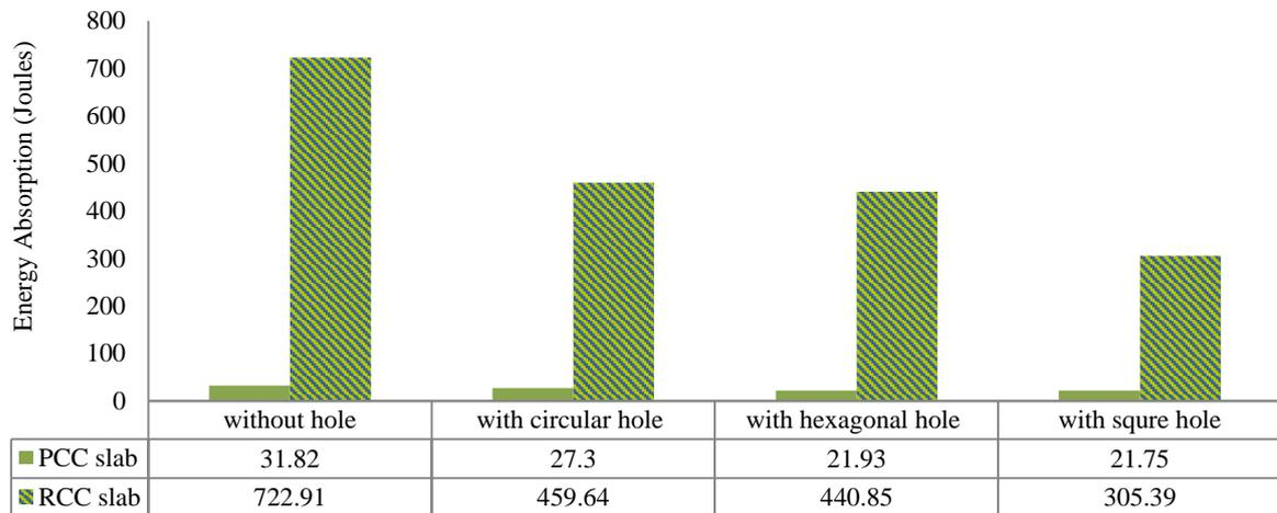
**Figure 7. Energy absorption.**
