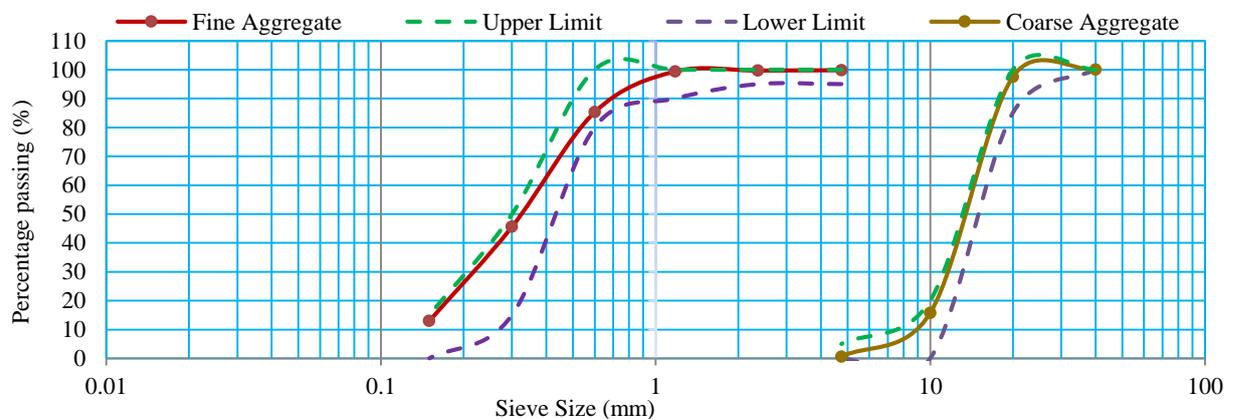
Figure 1. Particle size distribution of the aggregates.
