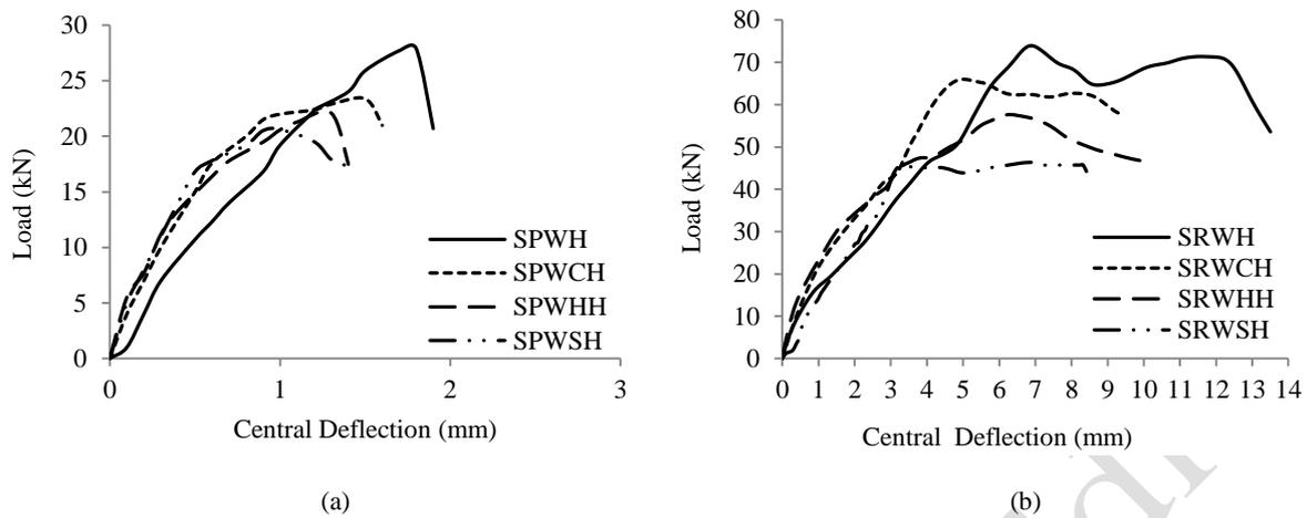
Figure 4 Comparison of load-displacement graphs of: (a) PCC Slab and (b) RCC slab.
