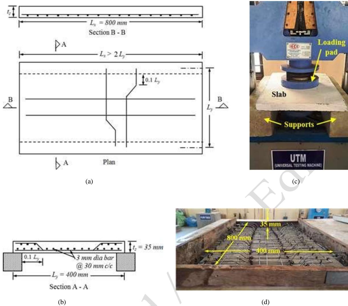
Figure 3. Graphical representation of reinforcement detailing and test setup.
