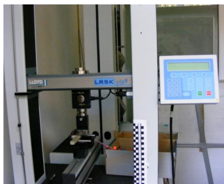
Fig 3: Bending machine inputs and outputs
