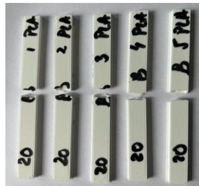
Fig 6: Orientation 45° for PLA samples, density 20%
