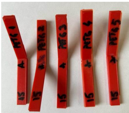
Fig 5: Orientation 0° for PETG samples, density 15%
