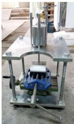
**Figure 3.** Cerchar abrasiveness testing device
