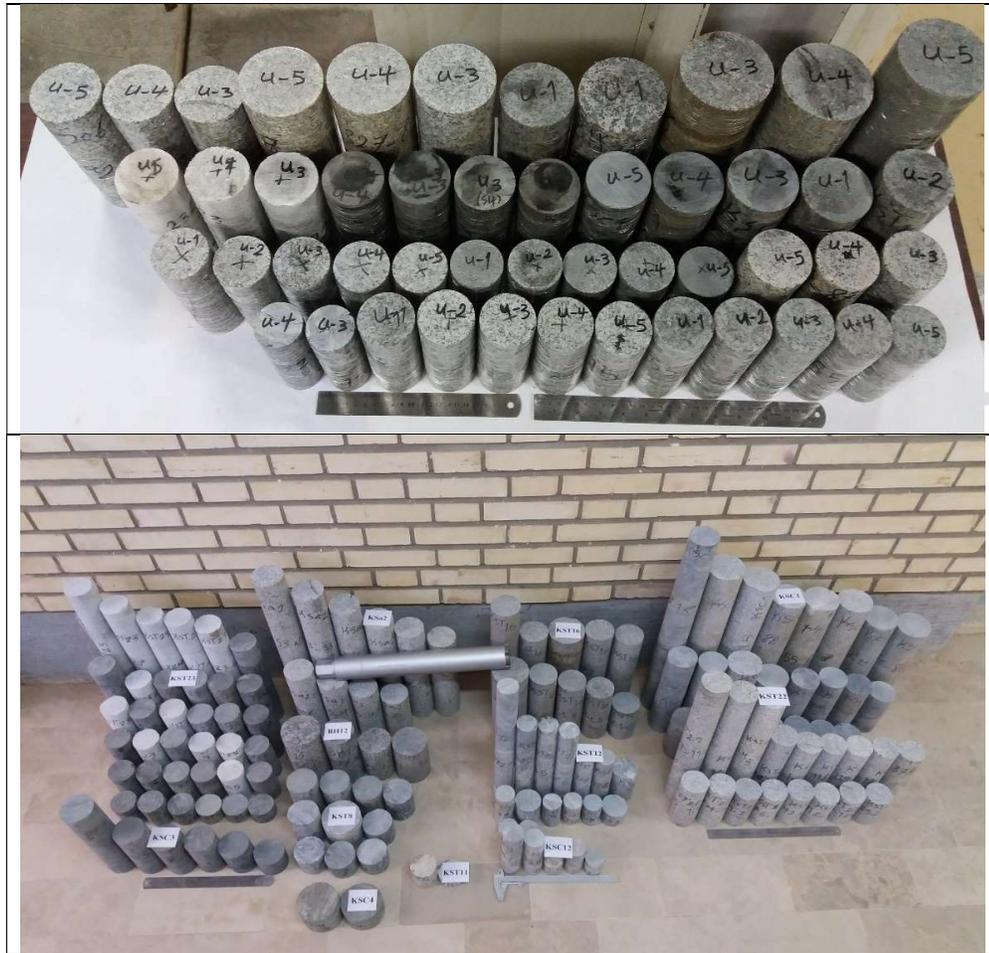
**Figure 2.** The picture of cylindrical cores rock samples
