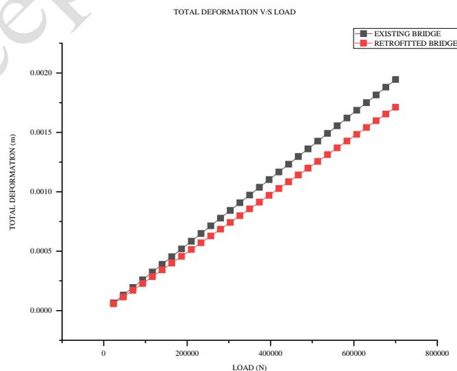
Fig. 4: Total deformation v/s load of existing bridge and retrofitted bridge
