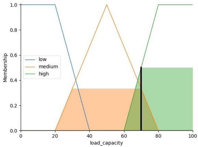
Fig. 14: Membership Functions for Load Capacity
