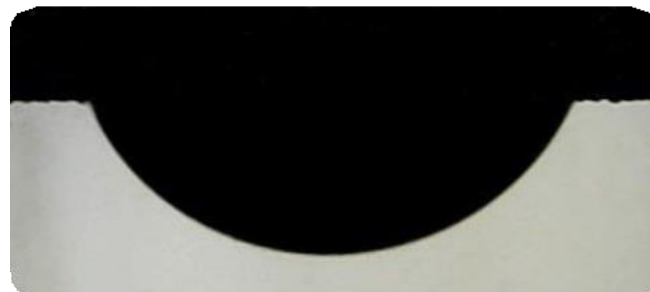
Fig. 5. Contact angle between rock and oil in the initial state
