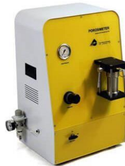
Fig. 2. A schematic of the helium porosimeter device
