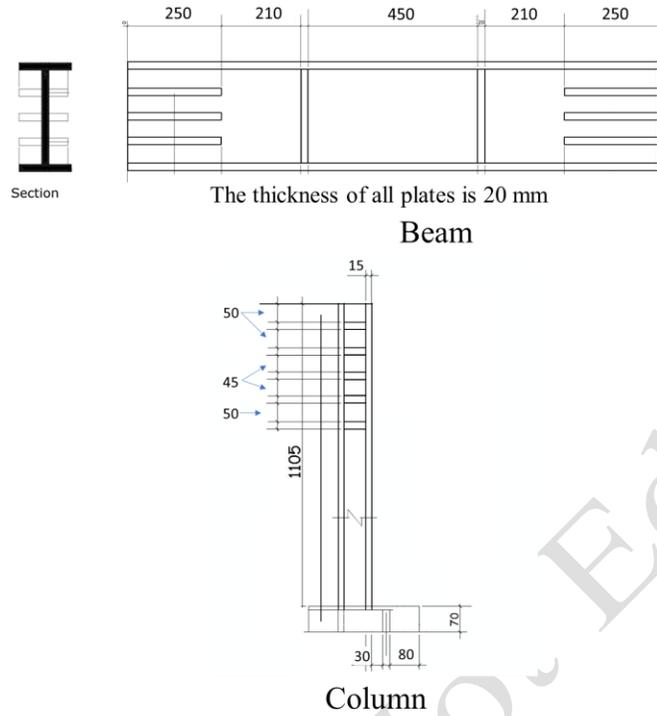
Fig. 2 Details of the beam and column (Units: mm)
