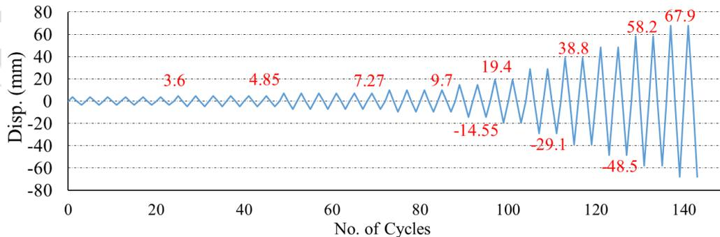
Fig. 3 The ASCE 7 loading protocol (ASCE, 2016).
