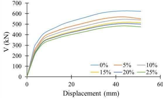
Fig. 13 Backbone curve for different openings.
