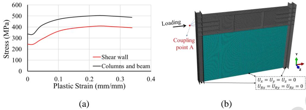
Fig. 8 (a) Material property (b) Boundary conditions of the numerical model.
