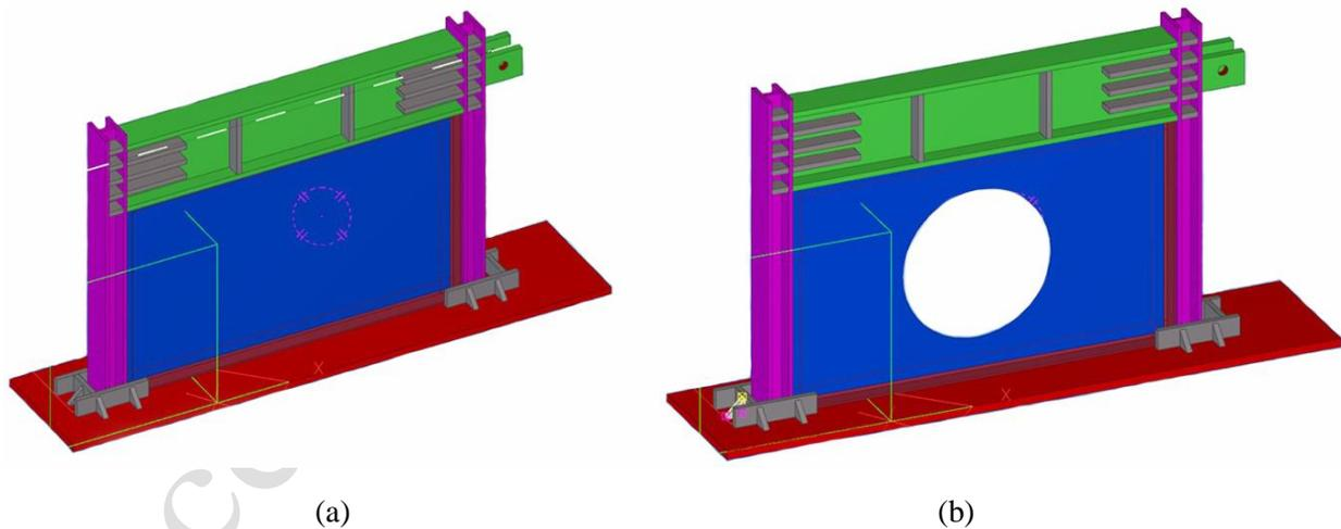
Fig. 1: Final design of the steel plate shear wall (a) without opening and (b) with opening
