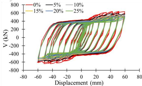
Fig. 12 Hysteretic curves for different opening configurations.
