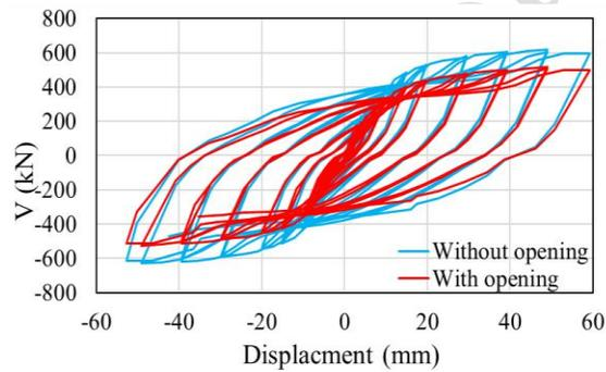
Fig. 6 Comparing the hysteretic curves of the two specimens with and without an opening.
