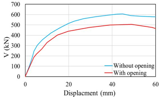
Fig. 7 Comparison between the backbone curves of the samples with and without an opening.
