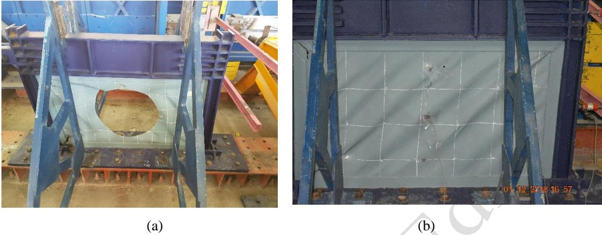
Fig. 5 Final loading cycle for the (a) sample with an opening and (b) without an opening.
