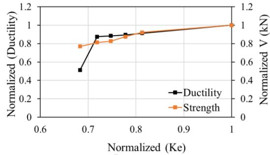
Fig. 18 The results of normalized ductility and strength versus normalized stiffness
