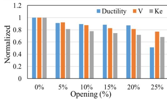
Fig. 19 The impact of the opening area on normalized results.
