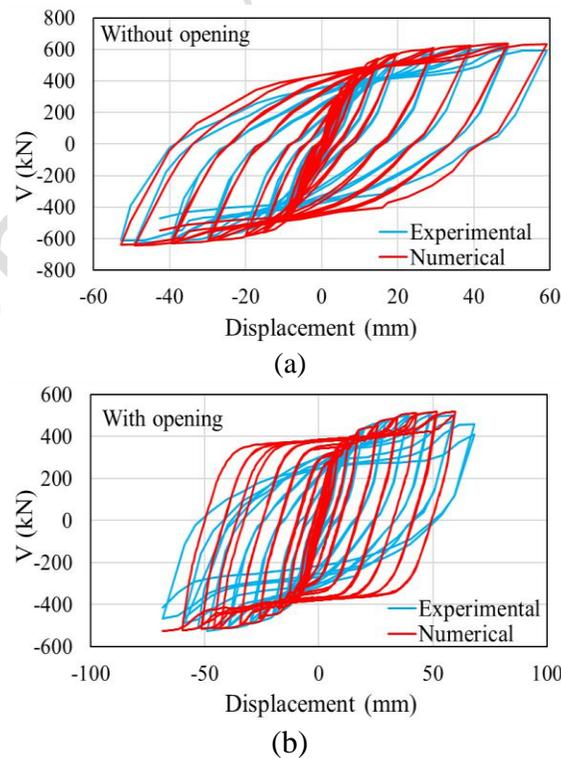
Fig. 9 Comparison of numerical and experimental results: (a) without openings, (b) with openings.
