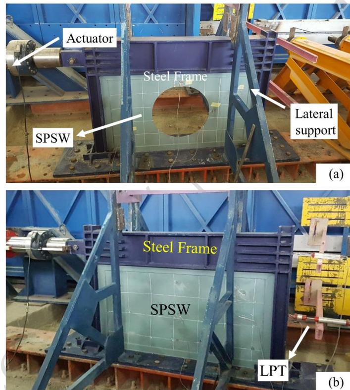
Fig. 4 Steel plate shear wall in the lab (a) with an opening and (b) without opening.
