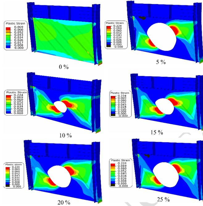
Fig. 11 Plastic strain contour results of models at different opening percentages
