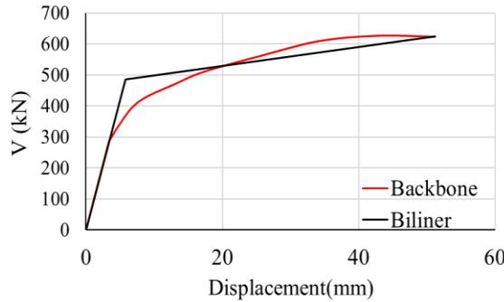
Fig. 14 Backbone and bilinear diagrams of the shear wall without an opening.
