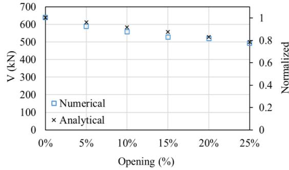
Fig. 15 Base shear relative to opening percentage.
