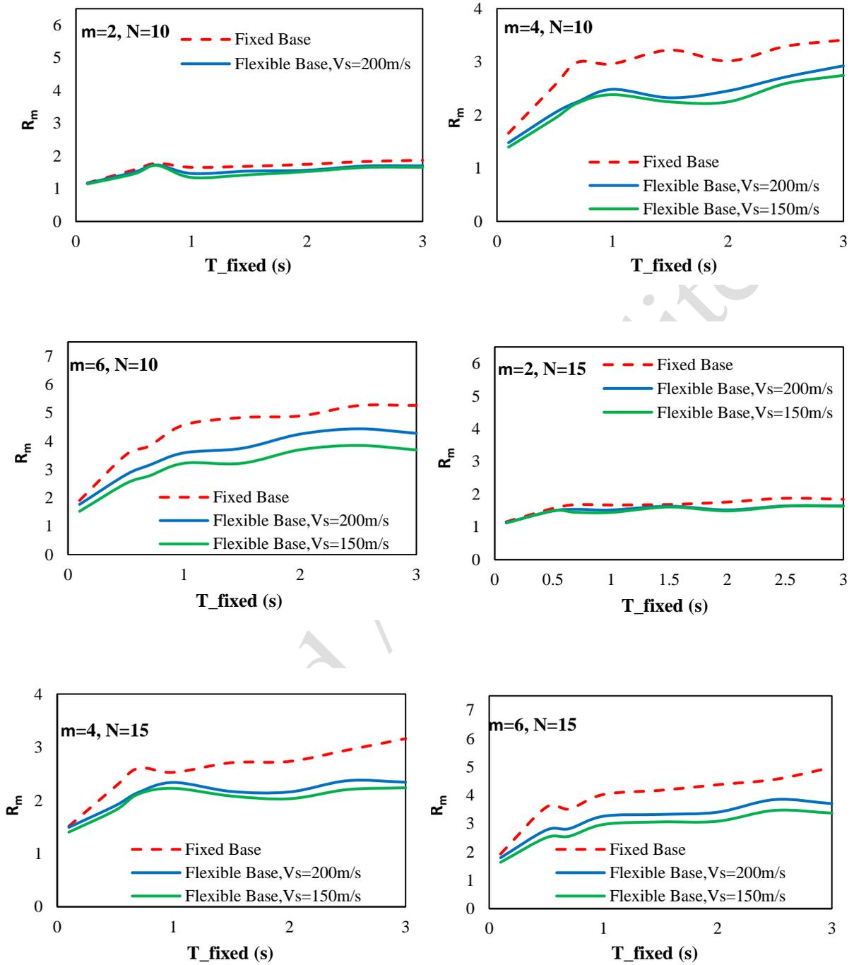
**Fig. 10. The effect of ductility demand ratio on Ductility Strength reduction factor for 3, 5, 10 and 15 story structures on soil type D and E**
