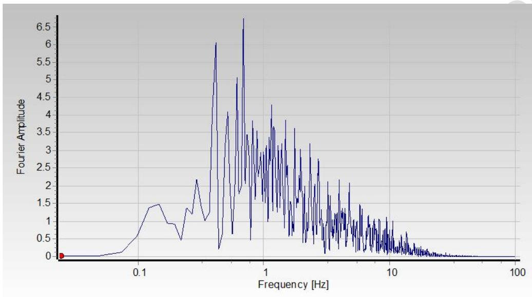
**Fig.5. Fourier spectrum of Imperial Valley earthquake ground motion**
