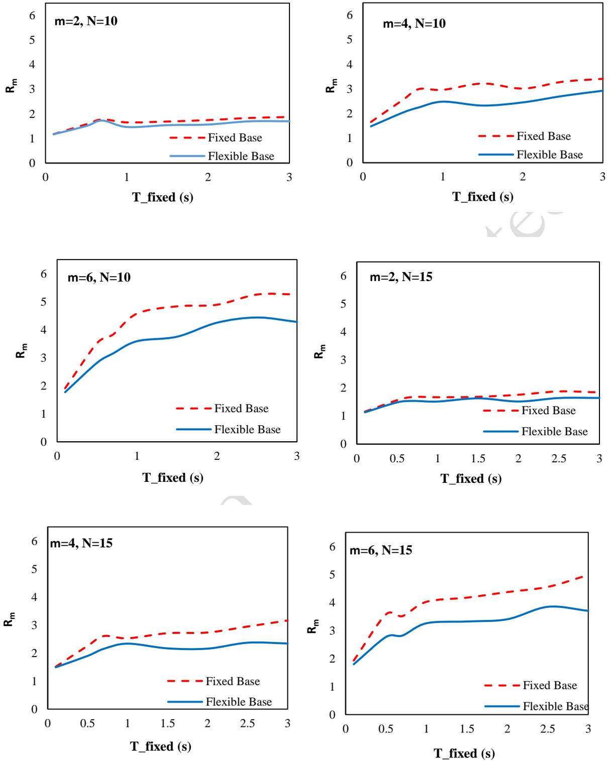
**Fig. 7. Strength reduction factor of fixed-base case and flexible-base case for 3, 5, 10 and 15 story structures on soil type D**
