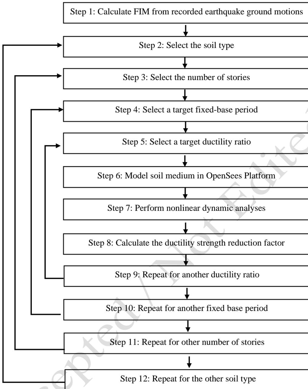
**Fig. 1. The diagram of creation the process of the new strength reduction factor formula**
