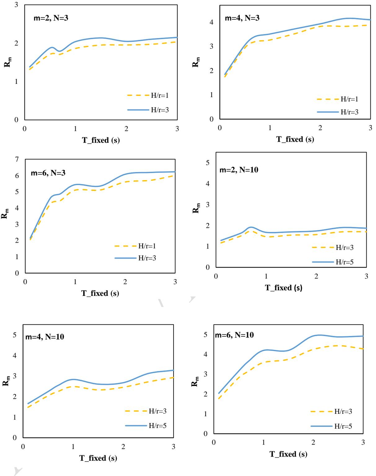
**Fig. 11. The effect of aspect ratio on Ductility Strength reduction factor for 3 and 10 story structures**
