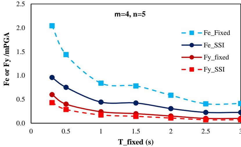
**Fig. 8. Elastic and inelastic strength spectrum of the soil-structure system on soil D compared to fixed-base condition**
