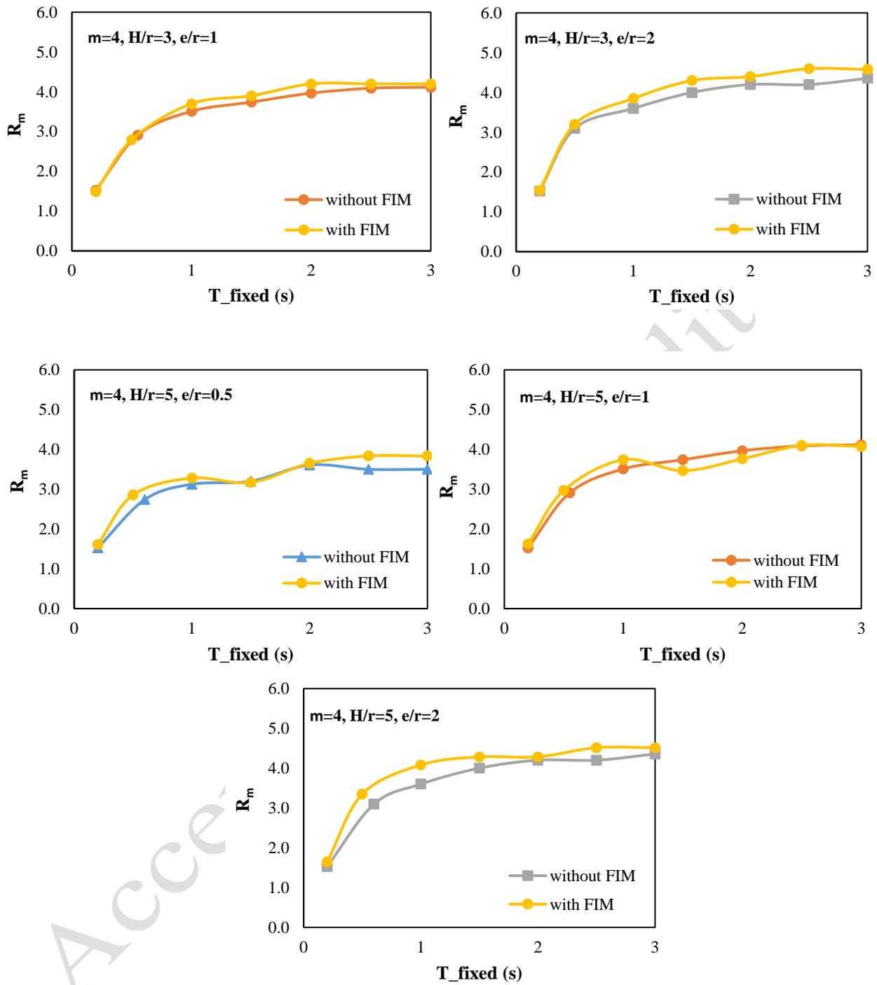
**Fig. 12.** The effect of kinematic interaction on Ductility Strength reduction factor for 10 story structures
