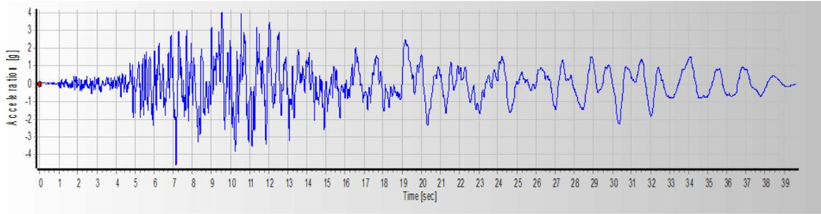
**Fig. 4. Acceleration time history of Imperial Valley earthquake ground motion**
