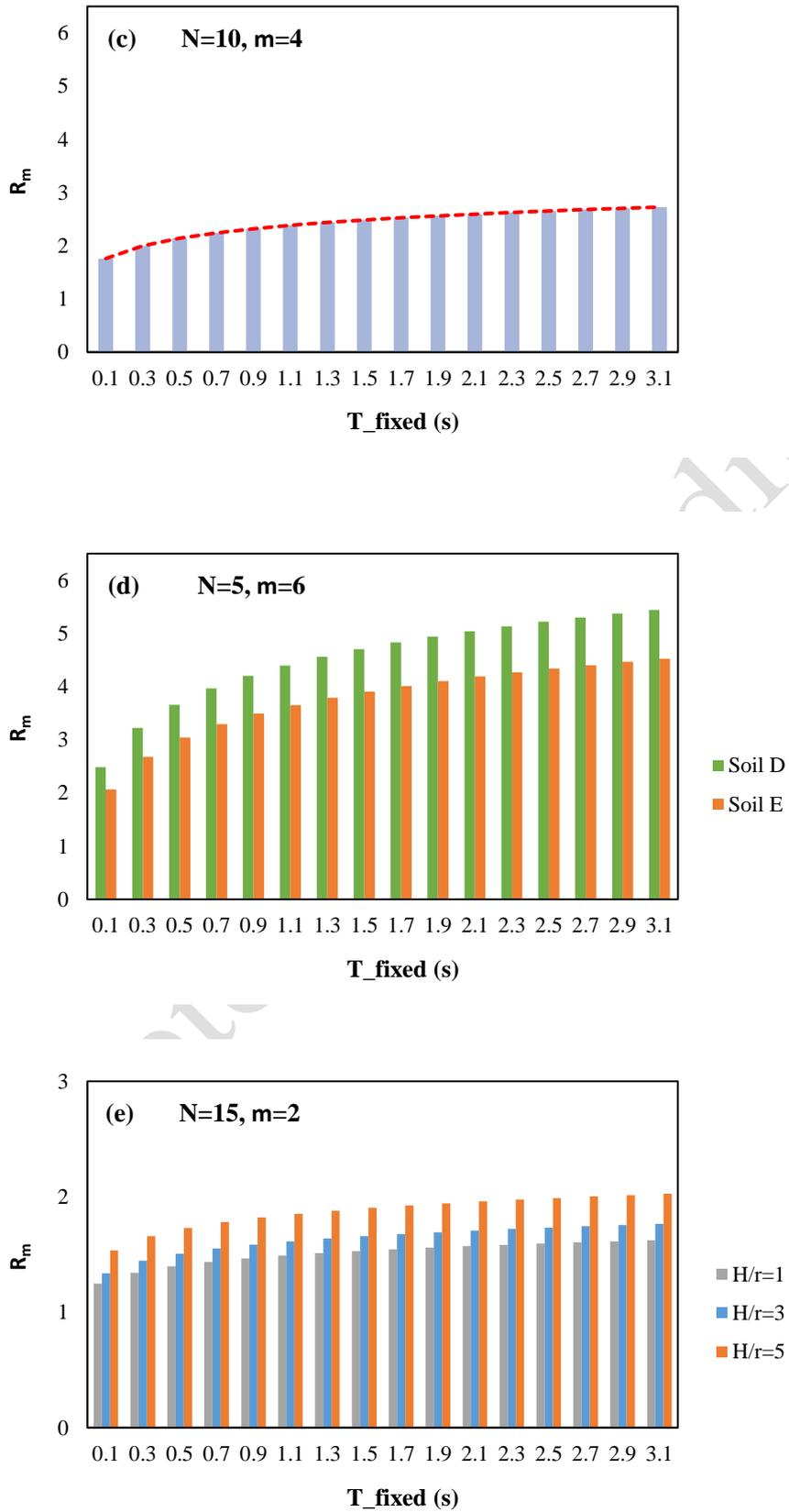
**Fig. 14. Sensitivity analysis of the ductility strength reduction factor compared to (a) ductility ratio, (b) number of stories, (c) fixed-base periods, (d) soil type and (e) aspect ratio**
