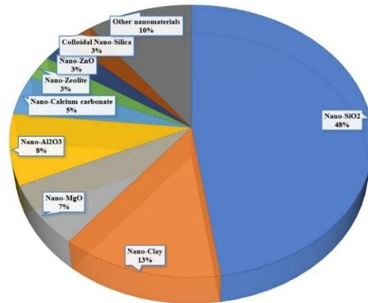
Figure 7. Distribution of nanomaterial types in soil stabilization
