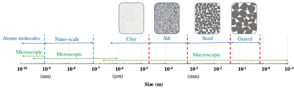
Figure 4. A comparative overview of soil particle sizes in relation to nanomaterial sizes
