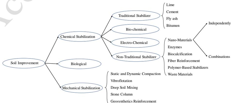
Figure 1. General soil stabilization methods
