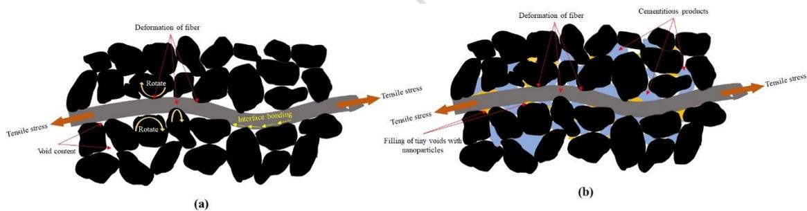
Figure 10. Schematic illustrating the contact conditions between soil particles and fiber: (a) without stabilizer, and (b) with stabilizer and nanomaterials.
