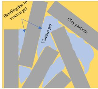
Figure 9. Formation of a viscous gel following the introduction of nanoparticles into cohesive soils
