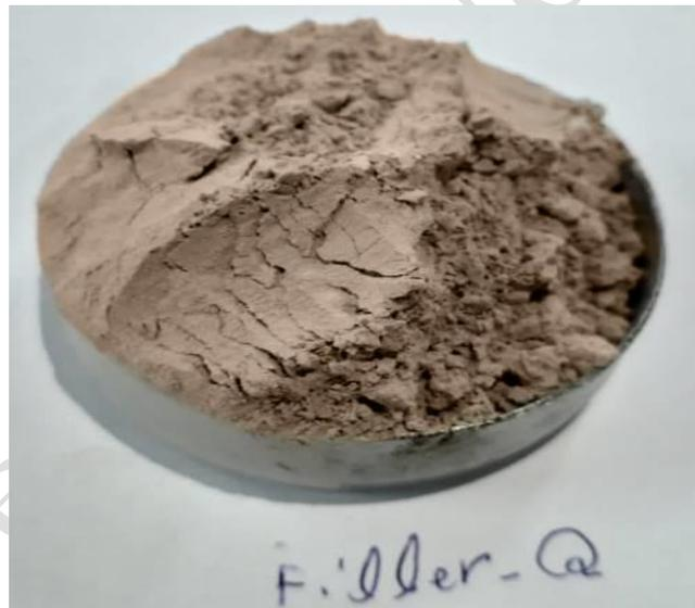
**Fig. 1: Photo of filler Limestone powder.**
