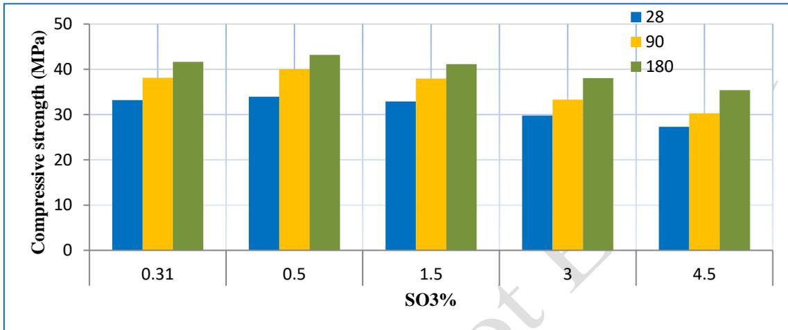
**Fig.5.** The impact of  $SO_3$  on compressive strength at (28, 90,180) days for LWSCC.
