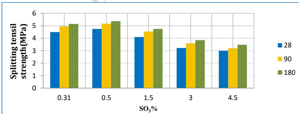
**Fig.8.**The impact of  $SO_3$  on Splitting-strength of NWSCC mixes at (28, 90,180).
