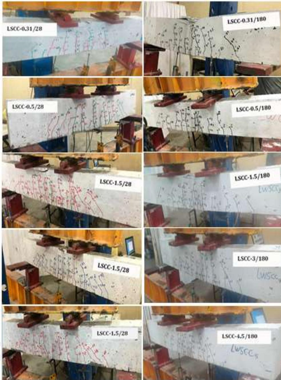
**Fig.10.** Crack pattern of LWSCC R.C. beams at 28 and 180-days tested.
