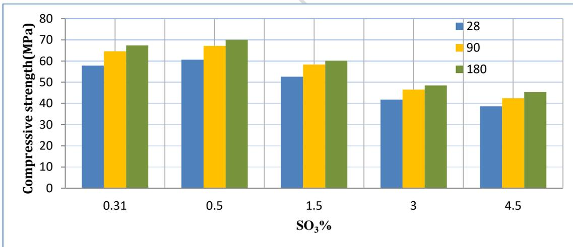
**Fig.6.** The impact of  $SO_3$  on compressive strength at (28, 90,180) days for NWSCC.
