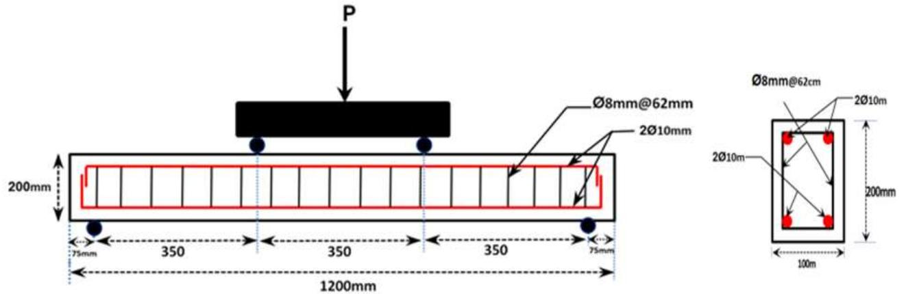
**Fig.2.** The Geometry of R.C beams samples and the arrangement of reinforcement configurations.
