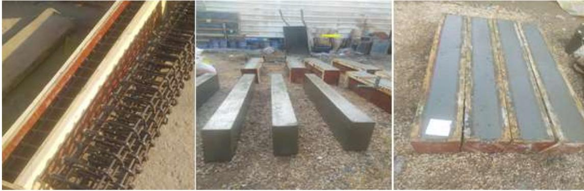
**Fig.3.** The preparation and casting of the R.C beam samples.
