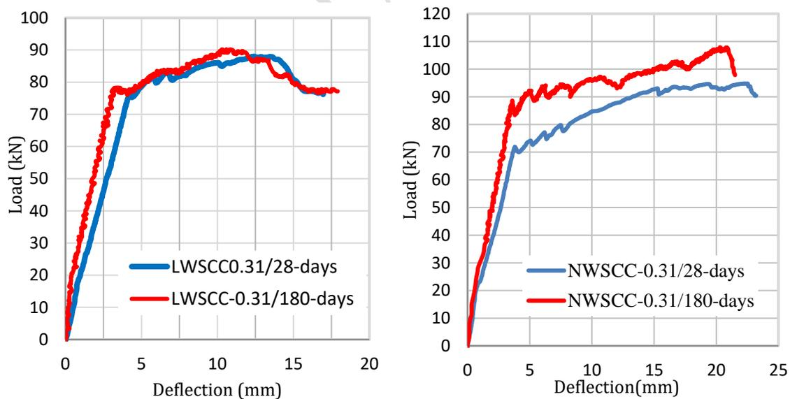
**Fig. 9.** The load-deflection curves for the tested R.C beams.
