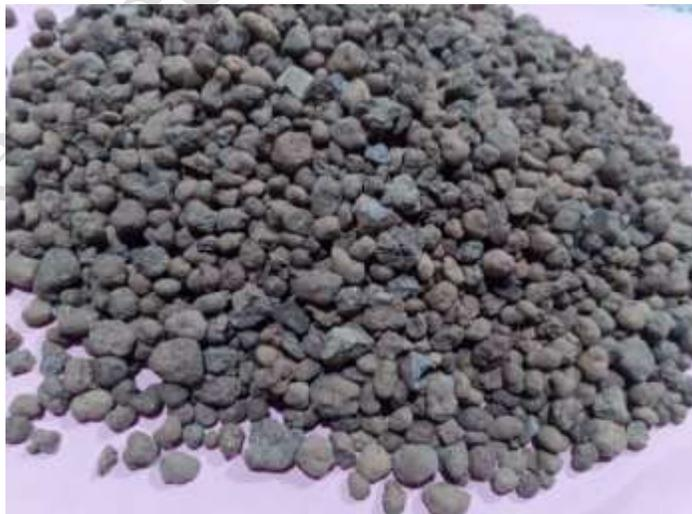
**Fig.1.** Lightweight expanded clay (LECA).
