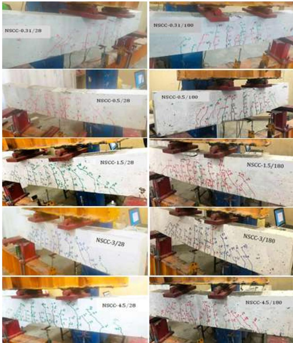
**Fig.11.** Crack pattern of NWSCC R.C. beams at 28 and 180-days tested.
