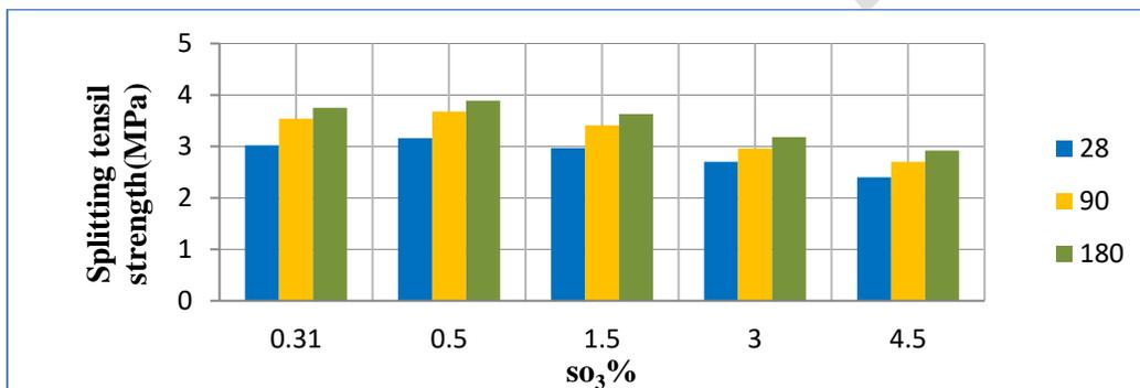
**Fig.7.**The impact of  $SO_3$  on Splitting-strength of LWSCC mixes at (28, 90,180).
